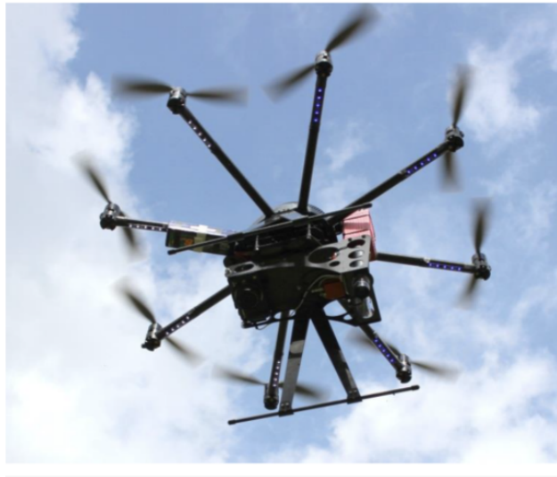
Figure 1.1: HYMSY hyperspectral sensor mounted on an Aerialtronics Altura AT8 v1 octocopter UAV [114]
