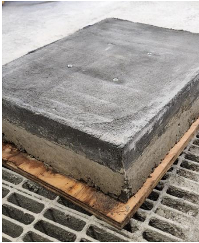
a) Cured slab before coring
