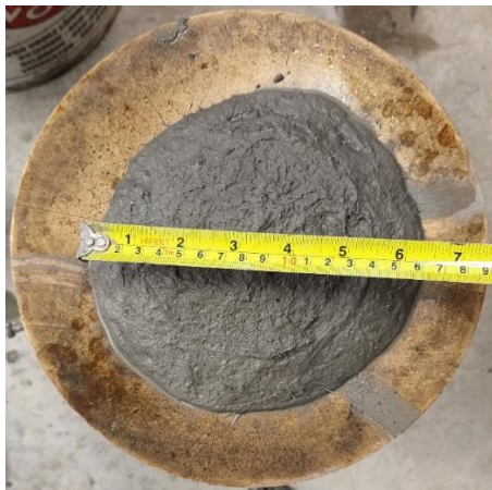
Figure 20: Dynamic flow test results for Ductal-T
