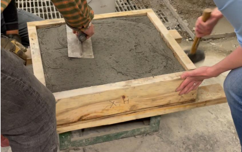
Figure 25: Typical consolidation process for thixotropic specimens including shake table (located below specimen form) and external tapping with rubber mallet
