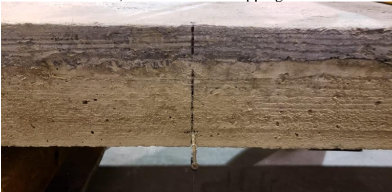
b) After UHPC chipping
