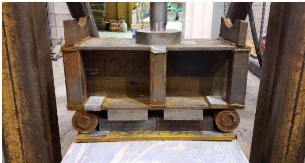
a) Load truck and steel plate
