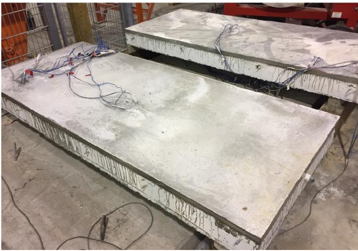
Figure 10: Example NC slabs with UHPC overlay and instrumentation [27]
