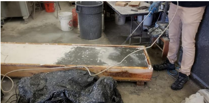
a) Spraying off curing compound
