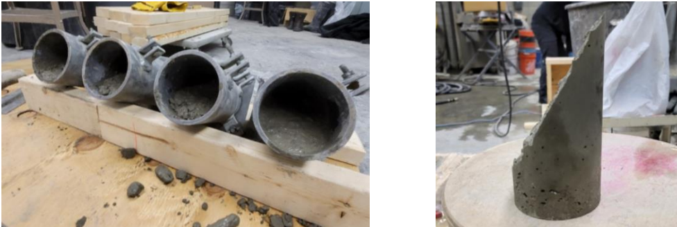
Figure 28: Typical substrate concrete half cylinders for slant shear specimens
