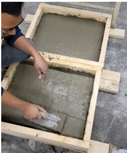
Figure 22: Typical substrate concrete slabs for direct tension specimens
