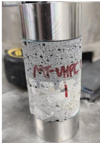
d) Core prepped for testing
