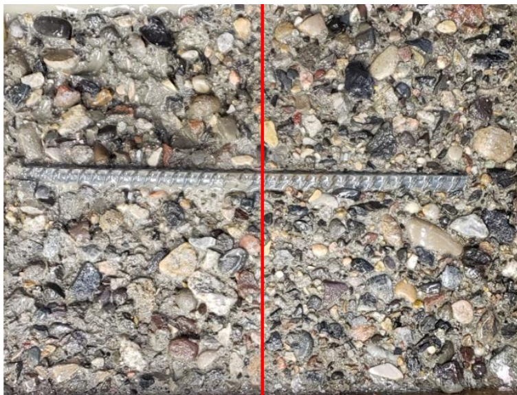
Figure 43: Hydrodemolition Test Slab (Left 7 hours. Right 20 hours)
