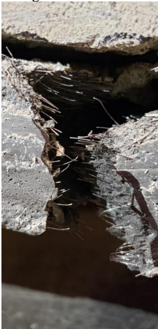
c) UHPC completely split
