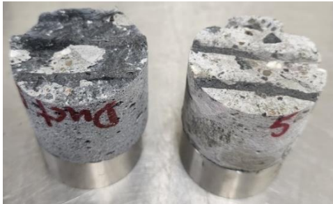
Figure 31: Example direct tension failure at the bond (Ductal-T Wet T1)
