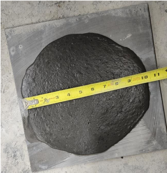
Figure 18: MT-UHPC static flow test
