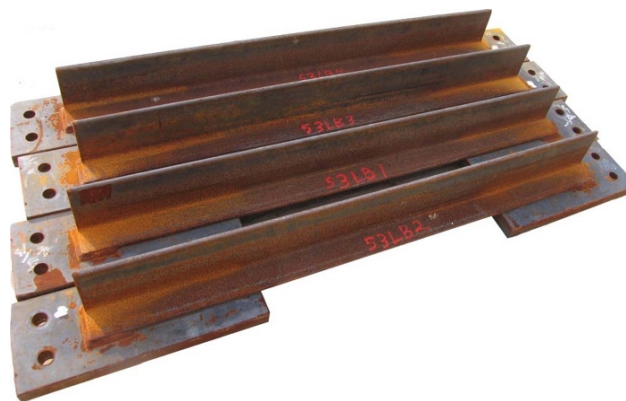
Figure 21. Angle-Plate Cross-Frame Specimens (McDonald and Frank 2009)
