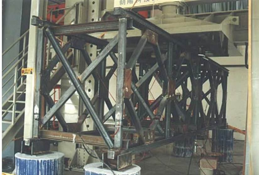
Figure 22. Full-Scale Bailey Bridge Model (King et al. 2013)
