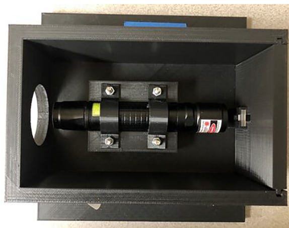
FIG. 2. Container and lens used to secure the laser and create a light sheet.
