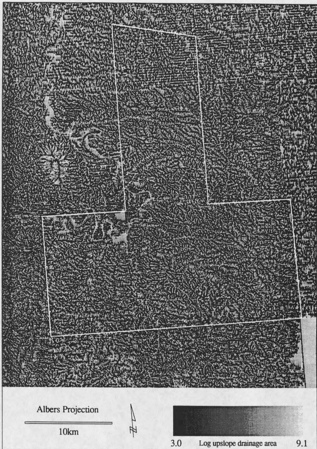
Figure 12. Upslope Contributing Area (sq. meters) Computed by TAPESG.
