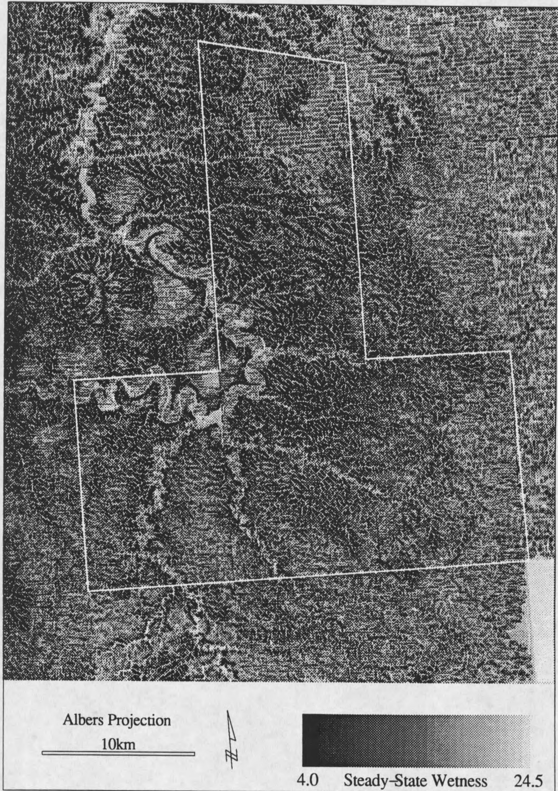
Figure 13. Steady-State Wetness Index Computed From TAPES-G Output.
