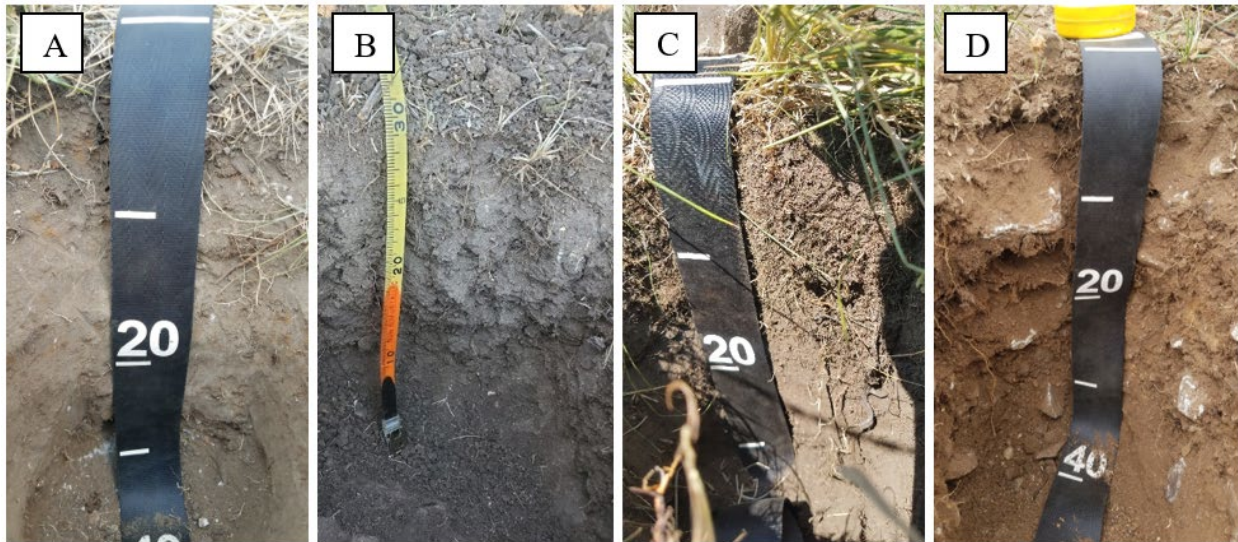
Figure 2-4: Representative soil pits at each catchment dug 30 cm deep 0.5 m upstream of lowermost structure or location in a reach. (A) Teepee Creek (TP); (B) Keystone Tributary (KEY); (C) Little Basin Tributary 7 (LB7); (D) Little Basin Tributary 24 (LB24)
