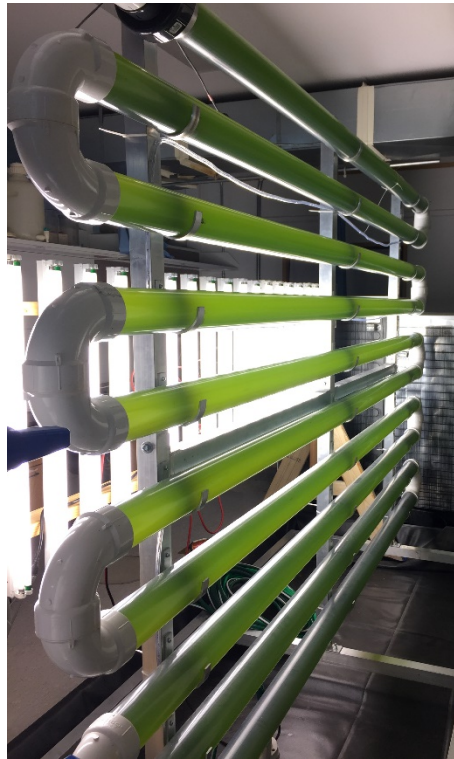
Figure 2.7 Photobioreactor illuminated (Green Wave Energy, Inc.) by artificial light in pilot-scale laboratory setting at Montana State University, Bozeman MT.
