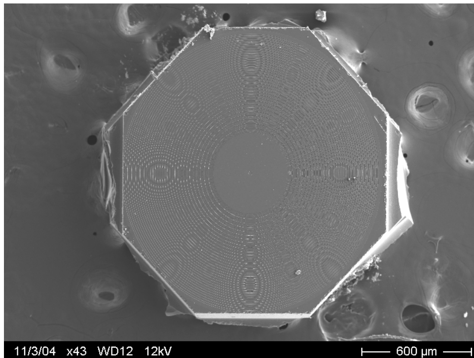
Figure 3.25: SEM of an 8-level DOE
