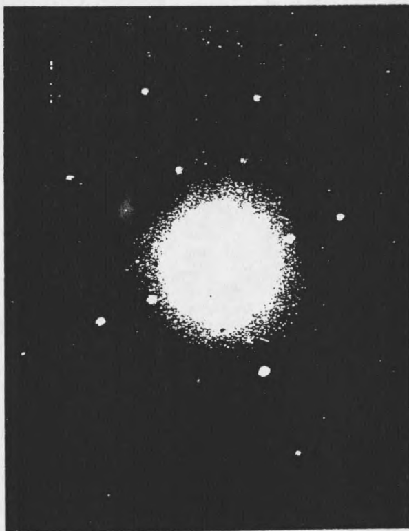
Figure 3.7 The Laue x-ray diffraction pattern from Al(110) single crystal surface
