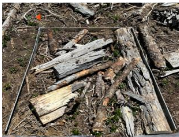
Sim. # 1, slashed tether road, 40% slope, 74 mm/hr rainfall Runoff ratio: 1%
