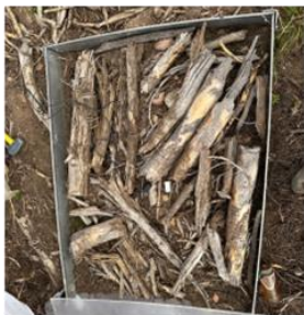
Sim. #18, slashed tether road, 20% slope, 74 mm/hr rainfall Runoff ratio: 4%
