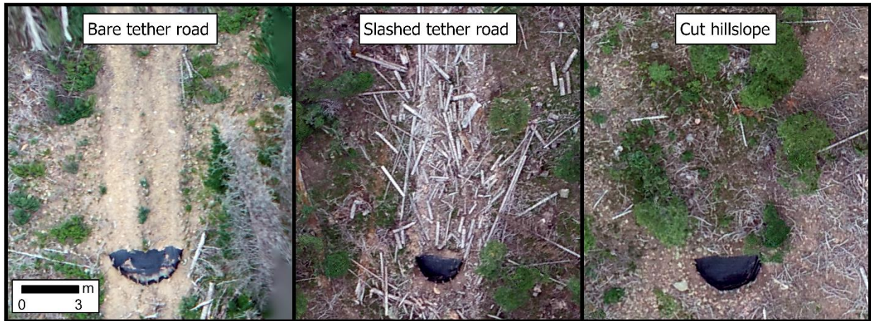
Figure 3. Drone imagery showing an example of a sediment fence installed in each ground cover treatment: (left) a bare tether road, (middle) a slashed tether road, (right) a cut hillslope in between tether roads. Drone imagery was acquired and processed by Dr. Peter Nelson, Colorado State University.
