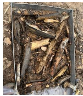
Sim. #16, slashed tether road 40% slope, 74 mm/hr rainfall Runoff ratio: 21%
