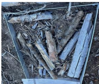
Sim. #8, slashed tether road 60% slope, 134 mm/hr rainfall Runoff ratio: 22%
