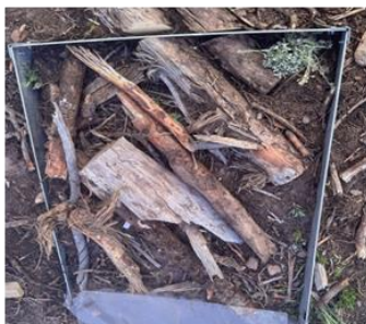
Sim. #2, slashed tether road 40% slope, 134 mm/hr rainfall Runoff ratio: 4%
