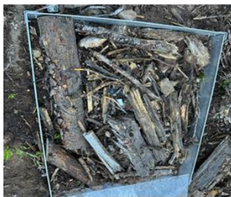
Sim. #7, slashed tether road 60% slope, 74 mm/hr rainfall Runoff ratio: 13%
