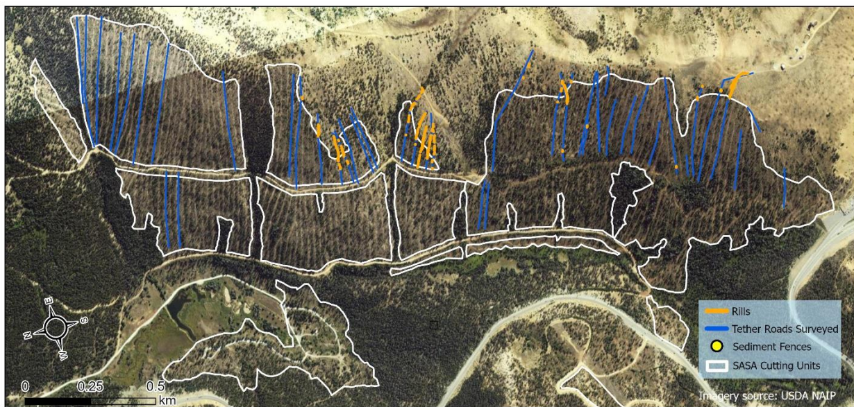
Figure 6. Map of rill surveys conducted in 2023. The orange lines show the rills identified on the tether roads while surveying and the blue lines show all the tether roads that were hiked. The ridgeline is located above the cutting units where the treeline is.
