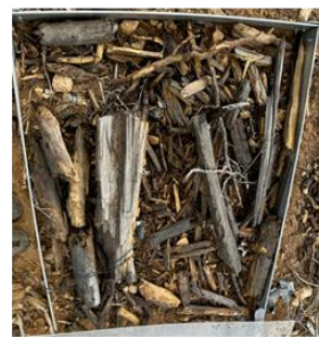
Sim. #14, slashed tether road 60% slope, 74 mm/hr rainfall Runoff ratio: 51%
