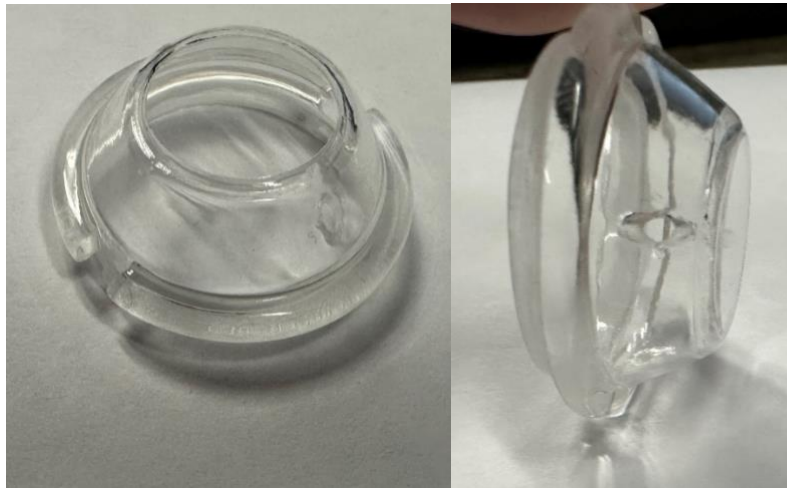
Figure 2.48. Window used by Caliber ID for imaging in clinical settings.
