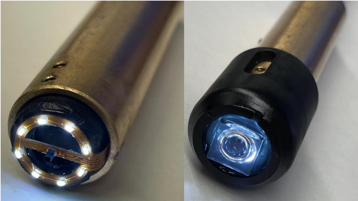
Figure 2.12. Populated flex board mounted to the adjustable 3D printed post inside a brass protective enclosure (left). Hyper-hemisphere approximation mounted to 3D printed objective and attached to the brass protective enclosure for imaging (right).
