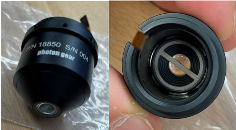
Figure 1.3. Objective lens housing partially assembled with flex board and hyper-hemisphere from Photon Gear Inc.
