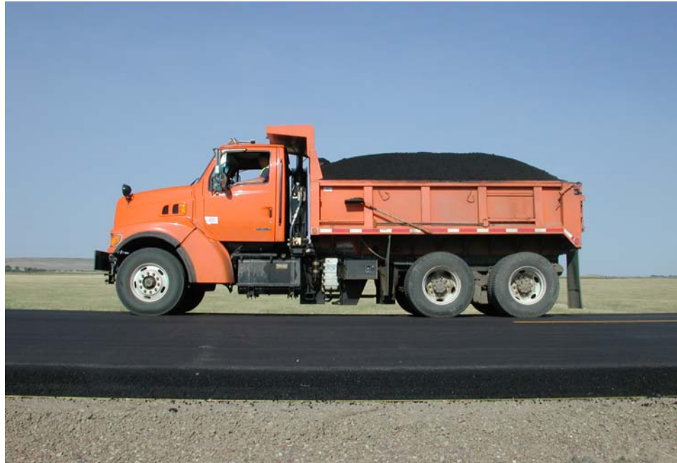
Figure 23 Side view of the Sterling 3-axle dump truck
