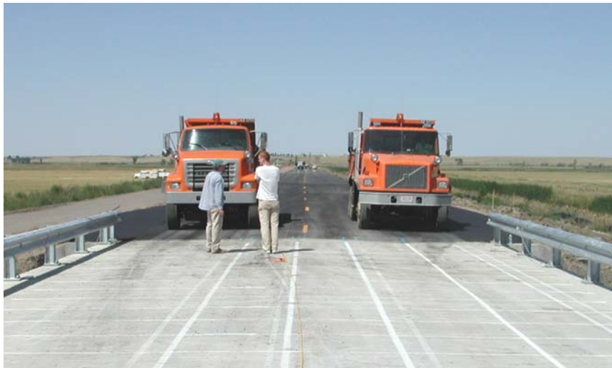
Figure 46 Test trucks preparing for a Two-Truck test
