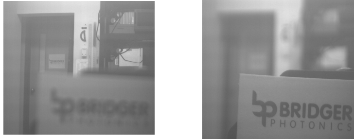
Figure 57. Left image, focus is at infinity. Right image, focus is on business card 126 mm away [65].
