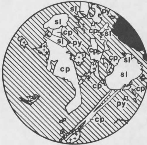
Figure 44. Relict grains of chalcopyrite (cp) and sphalerite (sl) in tetrahedrite (diagonal lines). Other components in the sketch are milky quartz (black), pyrite (py), and pits (+) in the sample. Sample S-23-27.6A. Diameter of field of view is 0.23 mm.
