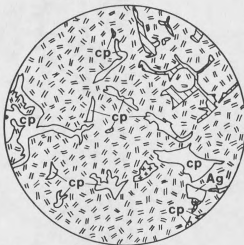
Figure 41. Grains of chalcopyrite (cp), tetrahedrite (diagonal lines), and silver (Ag) in bismuthinite (=). These grains suggest open-space or fracture filling perpendicular to the plane of the polished section. (+) is a pit in the sample. Sample S-41-24C. Diameter of field of view is 0.47 mm.
