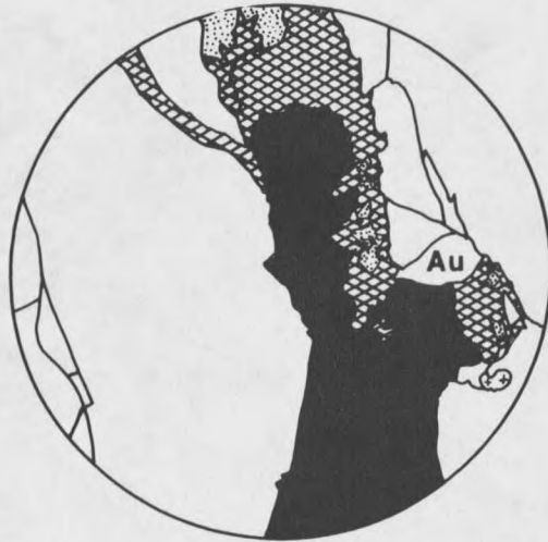
Figure 29. Gold (Au) localized along a fracture in pyrite (white). Additional fracture filling includes milky quartz (black), goethite (cross-hatched), and djurleite (dots). (+) is a pit in sample. Sample S-21-17.7. Diameter of field of view is 0.23 mm.
