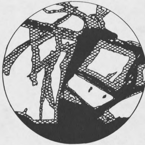
Figure 51. Replacement of pyrite (white) by goethite (cross-hatched). Milky quartz (black) is the matrix. Sample UW-1. Diameter of field of view is 0.47 mm.
