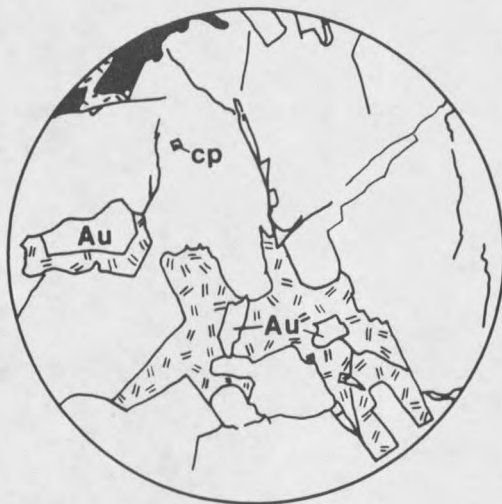
Figure 36. Bismuthinite (=) and gold (Au) in an open-space filling in pyrite. Mica (-) and milky quartz (black) bound pyrite. (cp) is a chalcopyrite grain in pyrite. Sample S-23-8. Diameter of field of view is 0.23 mm.
