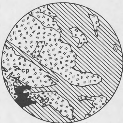
Figure 38. Relict grains of bismuthinite (=) in tetrahedrite (diagonal lines). Additional components in this sketch include milky quartz (black), chalcopyrite (cp) and pits in the sample (+). Sample S-23-27.6D. Diameter of field of view is 0.23 mm.
