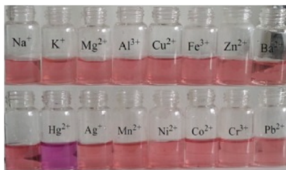
Figure 24. PODIPY 25 is a colorimetric sensor for \text{Hg}^{2+} , exhibiting a color change from pink to violet red. Reprinted with permission from [122]. Copyright 2015 Chinese Chemical Society and Institute of Materia Medica, Chinese Academy of Medical Sciences. Published by Elsevier B.V.
