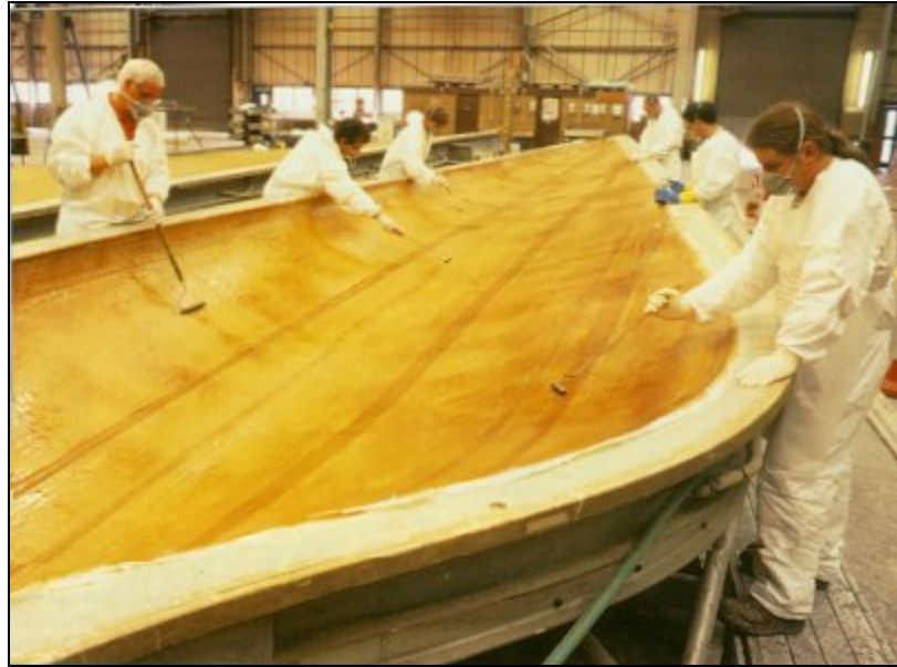
Figure 3: Physically laying up half a blade skin [5]
