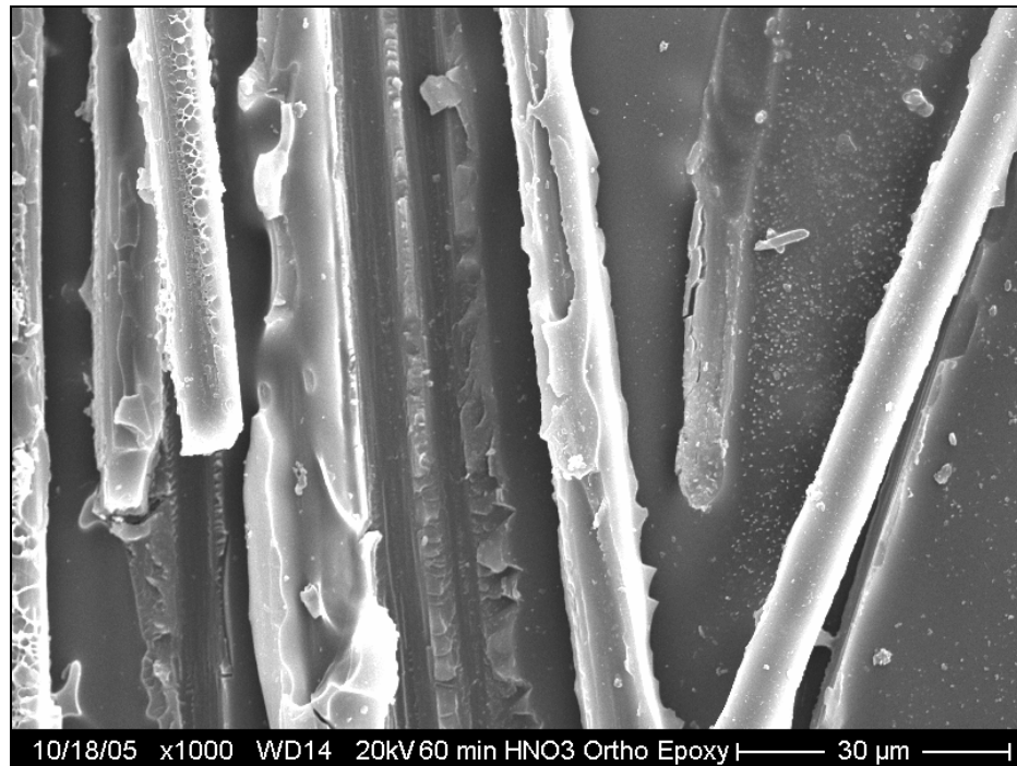
Figure H-33: Magnified view of post-tested secondary epoxy interface surface from unwashed 60 min \text{HNO}_3 treated rod with ortho spacing
