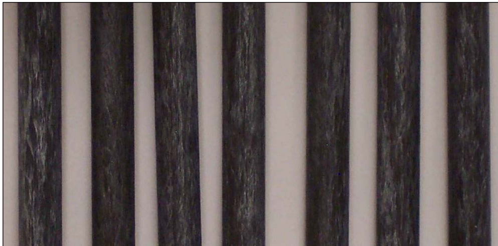
Figure 69: 30 min HNO 3 treated rod surfaces before secondary epoxy infusion
