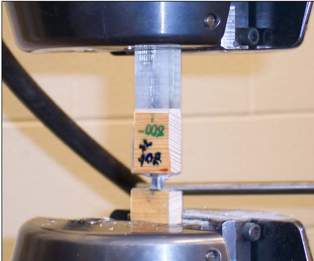
Figure 44: Pre-tested pullout coupon in grips
