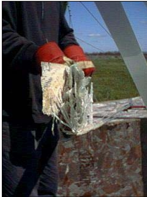
Figure 9: Straight on view of damaged blade [12]
