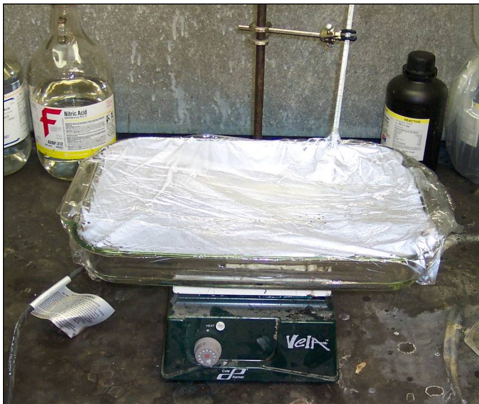
Figure 52: Heated nitric acid bath experimental setup
