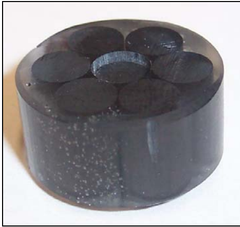
Figure 120: Typical pushout coupon interface failure appearance
