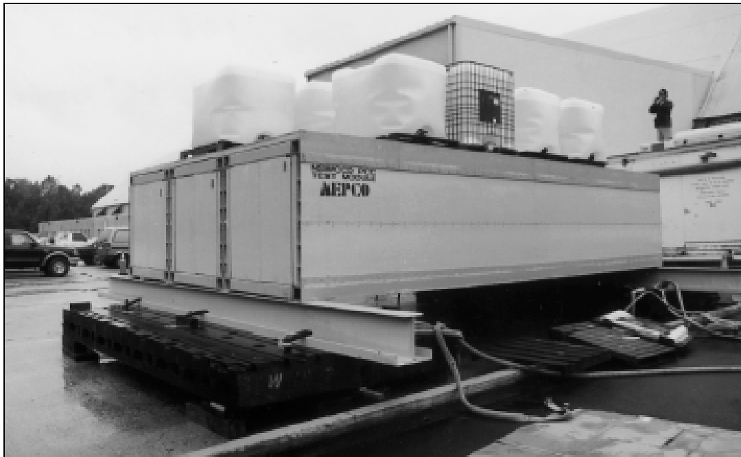
Figure 26: Completed causeway structure element under load [39]
