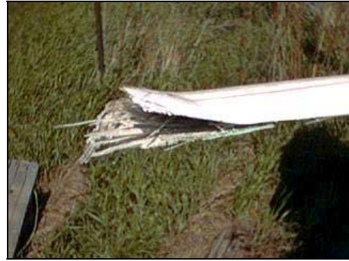
Figure 8: Same damage, view from trailing edge [12]
