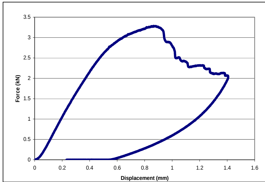
Figure 155: Typical force vs. displacement curve for a pultruded rod in short beam shear
