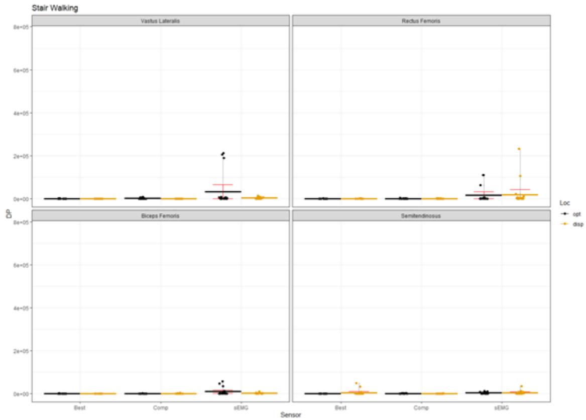
Figure 63: Violin graph of raw DP for Stair Walking. Opt is optimal placement, disp is displaced. Best (left) is Best Signal, Comp (middle) is Composite Signal, sEMG (right) is Traditional sEMG. Note presence of outliers for Vastus Lateralis (top left) and Rectus Femoris (top right).
