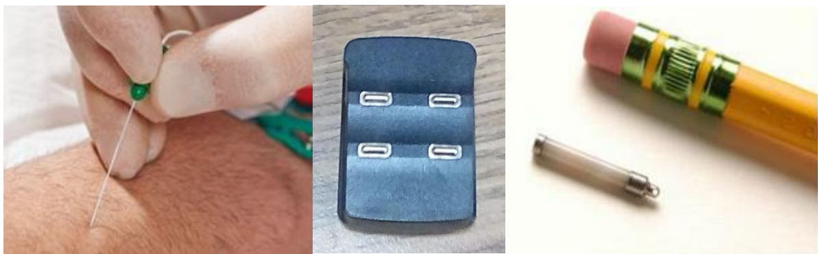
Figure 4: nEMG electrode (left 32 , Traditional sEMG electrode (center, picture by researcher), and IMES electrode (right) 29 Each type has advantages and disadvantages that must be considered before use
