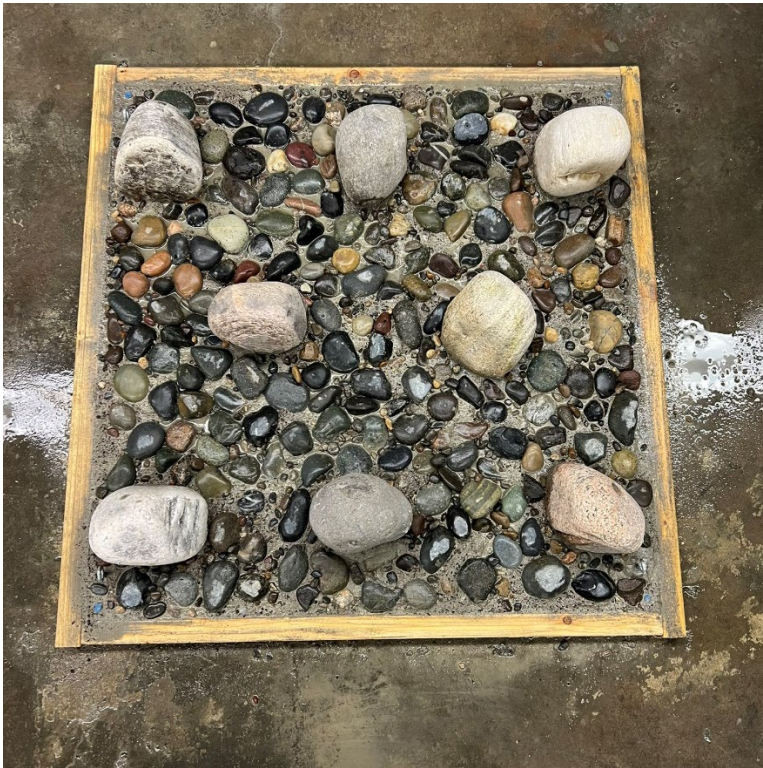
Figure 3: Rock ramp panel post construction including hardware, forms, perturbation boulders, and gravel substrate.
