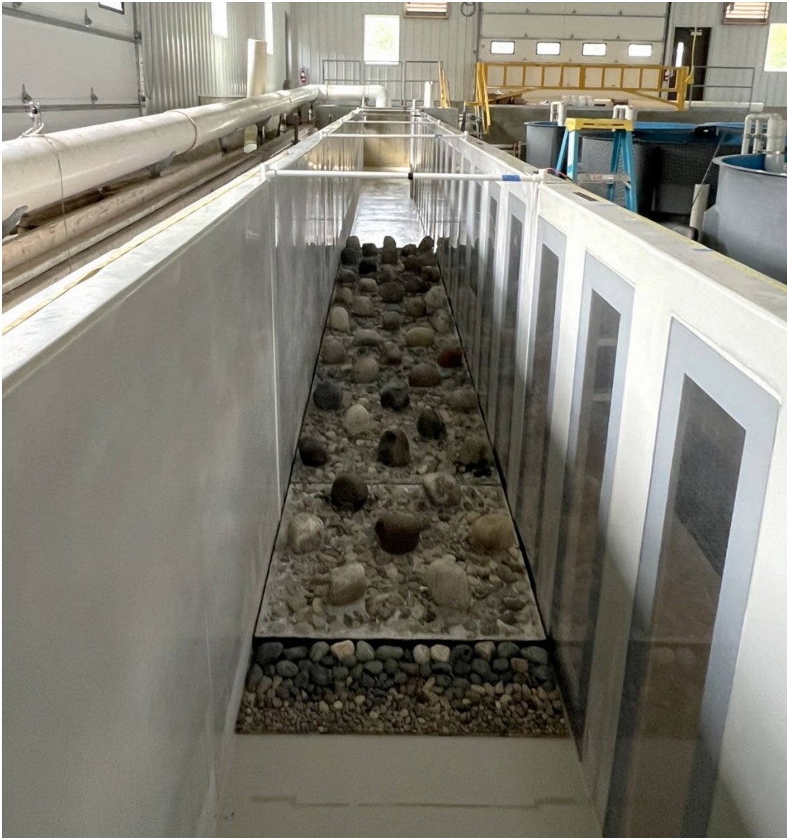
Figure 7: 3% slope rock ramp installed in flume looking upstream.
