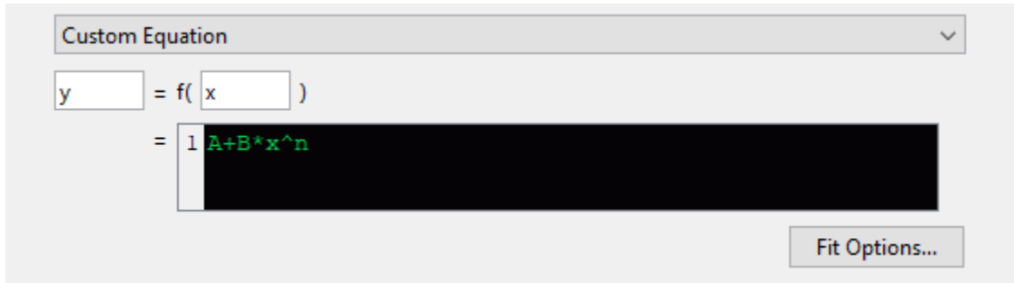
Figure 20. MATLAB Curve fitting app, A is filled with each test's respective yield stress value, B and n are solved for.
