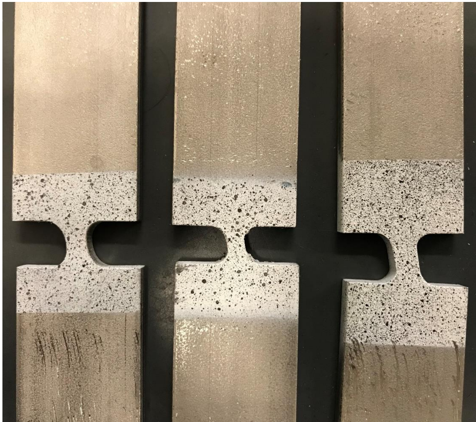
Figure 24. Desirable stochastic spray pattern on 304 stainless steel.
