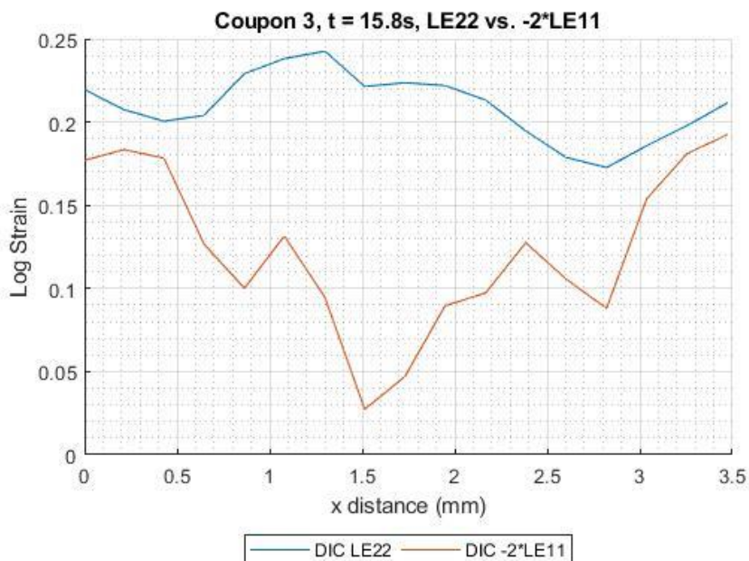
Figure 76. Plot comparing strain in the \epsilon_{22} direction against -2*(\epsilon_{11}) . t = 15.8s .
