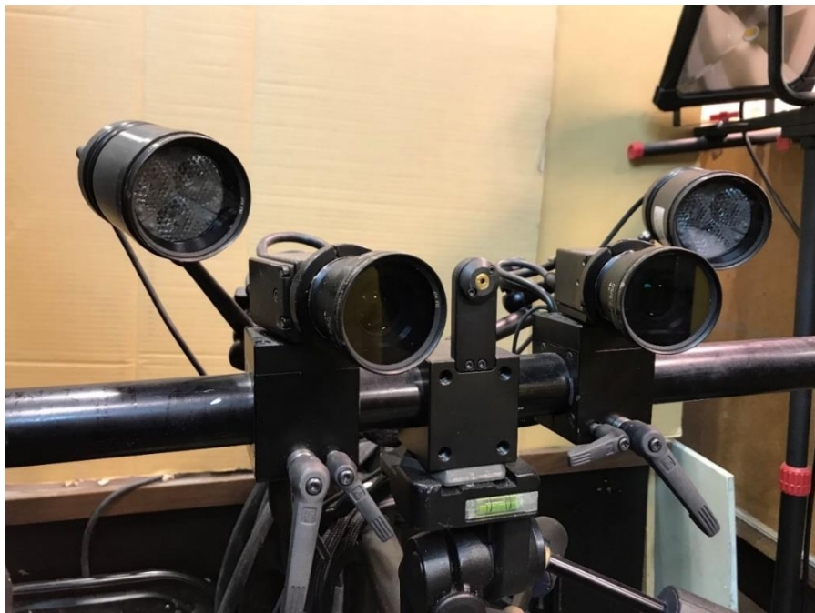
Figure 23. GOM designed camera set up used for IPL testing; cameras are mounted at a set distance from one another. Lighting elements can be adjusted for optimum position.
