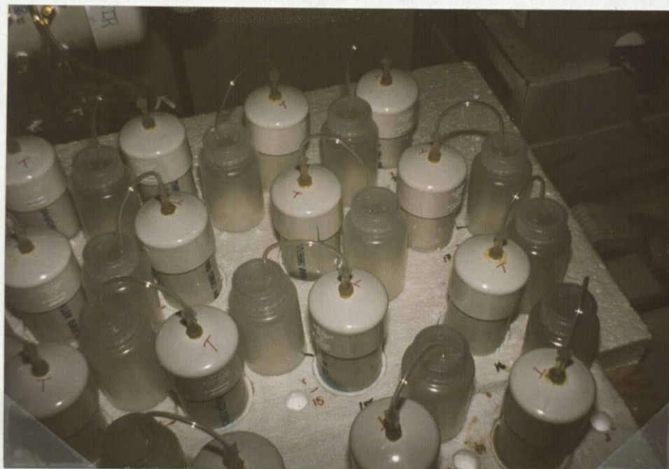
Figure 3. Polypropylene bottles (250 mL) were placed next to chambers to collect leachate during flushing cycles. Leaching solutions were pumped up through the chambers and collected in the bottles .
