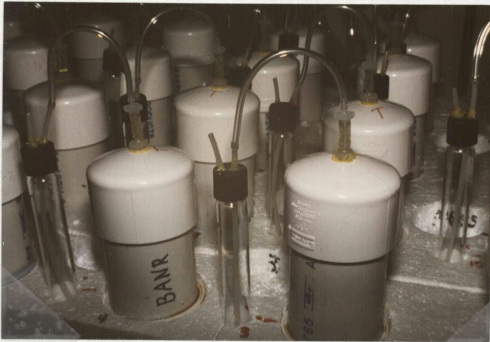
Figure 1. Incubation chambers with CO 2 -trap system attached. Air passes through the chamber and is directed to 25 mL test-tubes containing 20 mL of 0.5M NaOH where CO 2 is stripped from the air.
