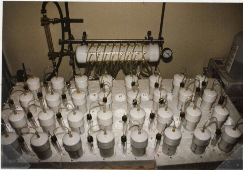
Figure 2. The thirty-two incubation chambers were placed on an incubation stand. Air manifold in background distributed compressed air to each chamber during incubation.
