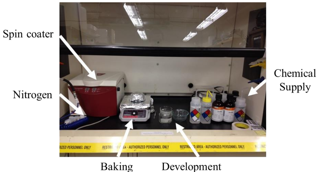
Figure 2-3. The in-lab photolithography and soft lithography station is housed in a fume hood. It consists of a spin coater, a nitrogen source, a baking unit, a development unit, and various chemical supplies.
