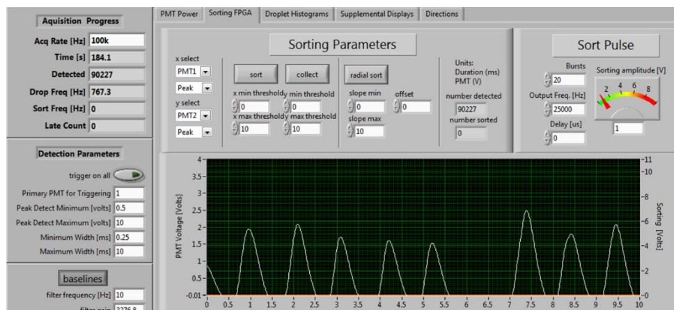
Figure 3-18. A screenshot of the LabVIEW interface during drop detection. Local peaks indicate the fluorescence within a drop is being detected. The magnitude of the peak is determined by the emission intensity.
