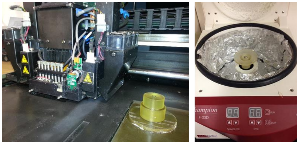
Figure 2-4. The 3D printed spin coater "chuck" and its assembly onto the centrifuge rotating shaft.
