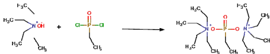
Figure 2.3: Synthesis of Bis(tetraethylammonium) ethylphosphate. A 40 % Tetraethyl ammonium solution was reacted with dichloro-ethyl phosphate to yield the desired product. (Kluger, et al. , 1996)
