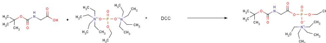
Figure 2.4: N-boc glycine was activated with DCC in dry DCM. Upon activation, Bis(tetraethylammonium) ethylphosphate was reacted with the activated N-boc glycine in order to form N-boc glycyl ethylphosphate tetraethylammonium salt (Kluger, et al. , 1996)
