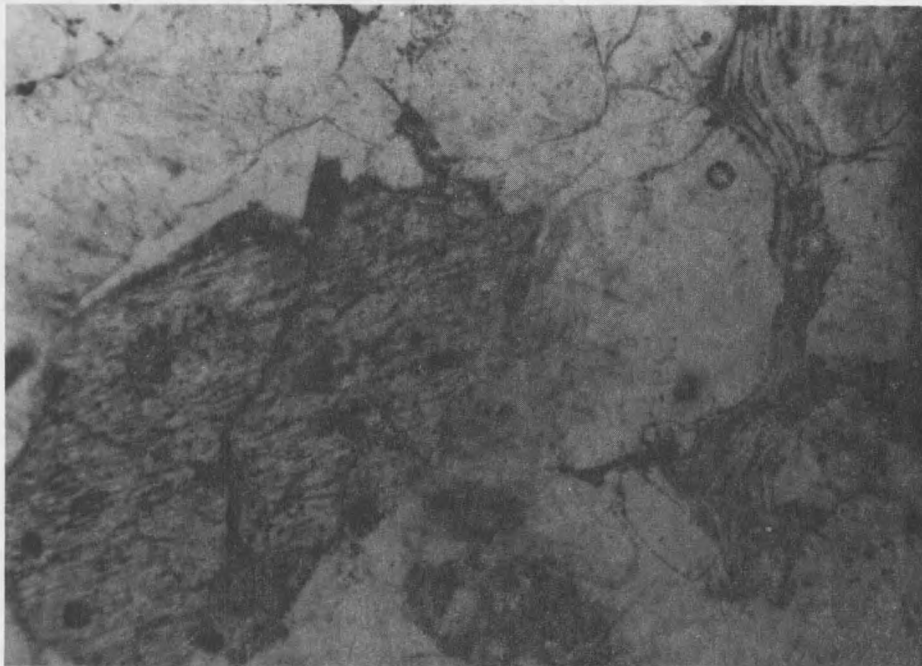
Figure 22. Large potassium feldspar grain altering to clay. Long muscovite grain (at right) has been deformed by quartz grains. Sample shows almost complete development of quartz overgrowths. Sample is from Birch Creek Section.
