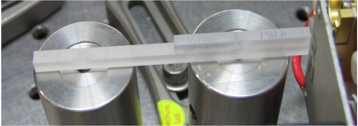
Figure 24: Mounting Method for Monoblock Interferometer Tests
