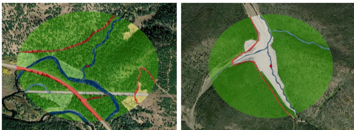
Figure 3.3. ArcGIS Buffers to Quantify LULC. 500-meter radial circles surrounding reference site Ref.ARC1 (left) and restored site Rest.BT2 (right). The area inside of the circle was characterized as coniferous/herbaceous vegetation (dark/light green), developed land/bare ground (red/tan), and river/side channels (dark/light blue).
