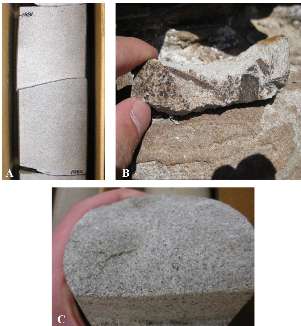
Figure 18. Massive sandstone in core R362 (A & C) and from outcrop with carbonaceous plant material (B) near Ryan Dam.
