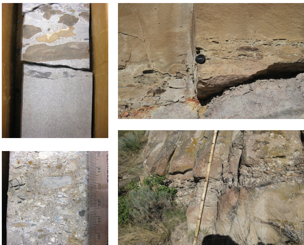
Figure 13. Conglomerate in core R362 and in outcrop near Ryan Dam northeast of Great Falls, MT.
