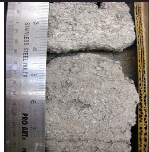
Figure 26. Alluvial plain system deposits found in outcrop near Ryan Dam. The coastal plain – estuary system is broken into two distinct facies associations flood plain deposits and channel deposits.
