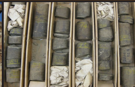
Figure 23. Fluvial channel fill in outcrop near Ryan Dam and in core R685. Intraformational flattened shale-clasts near the base of trough cross-stratified cosets and trough cross-stratified sandstone is observable in this FA.
