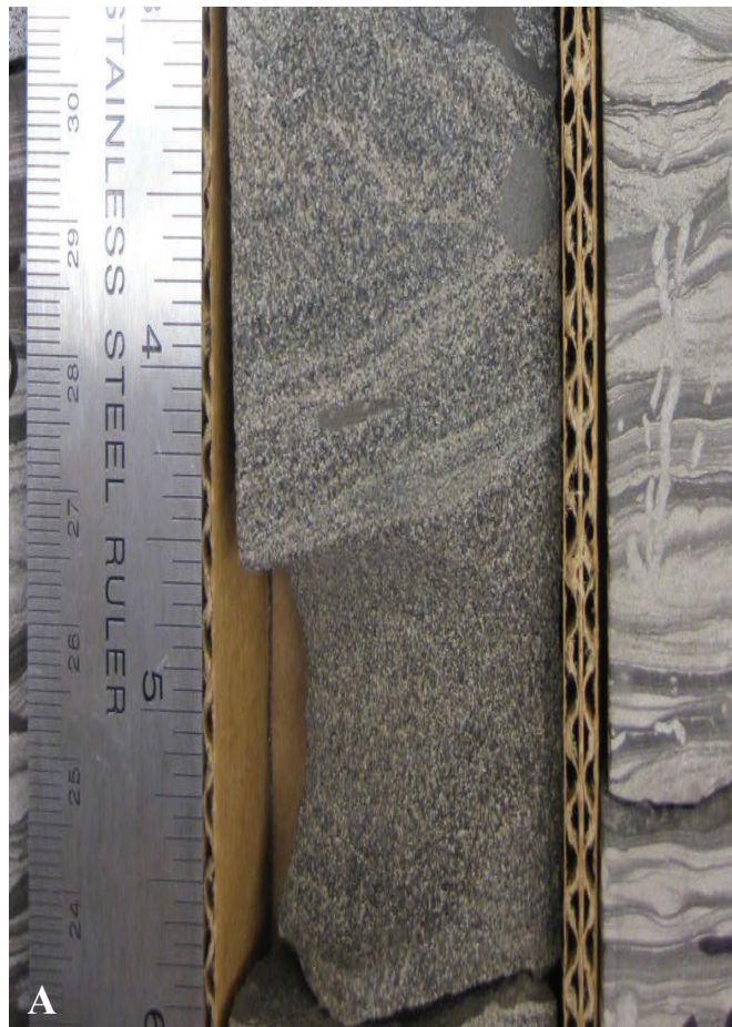
Figure 14. Trough cross-bedded sandstone in core E891
