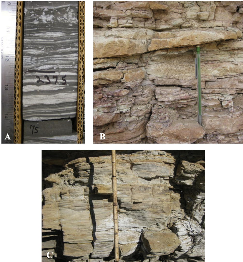
Figure 19. Interbedded heterolithic strata in core E891 (A) and in outcrop near Morony Dam (B) and near Ryan Dam (C).
