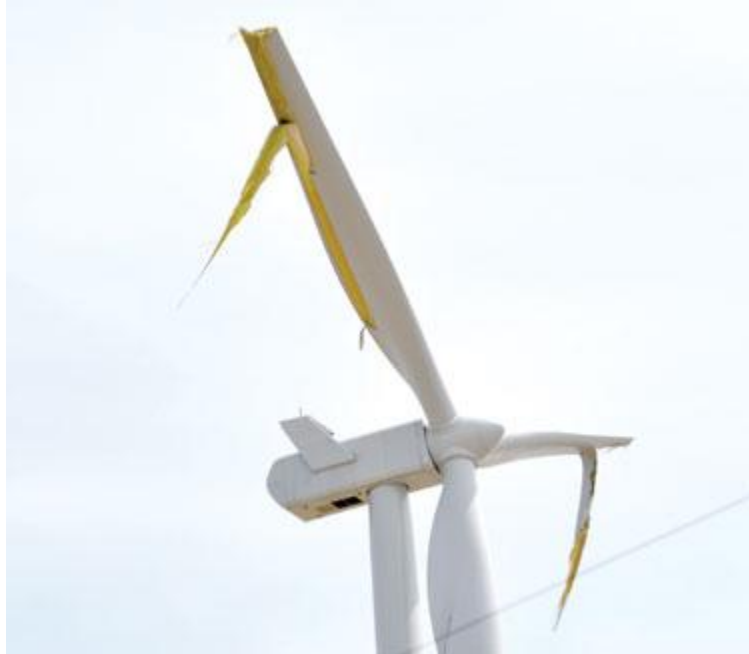
Figure 13: Wind turbine blades manufactured by Vestas which suffered failure due to manufacturing defects, [25].
