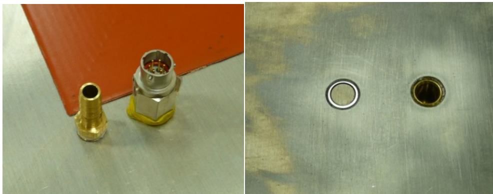
Figure 27: Mounting the transducers to the aluminum mold.
