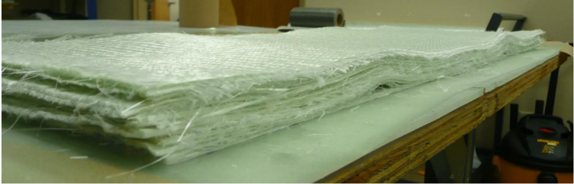
Figure 51: Out-of-plane waves inserted into 20 layers of uni-directional fabric using Super 77.
