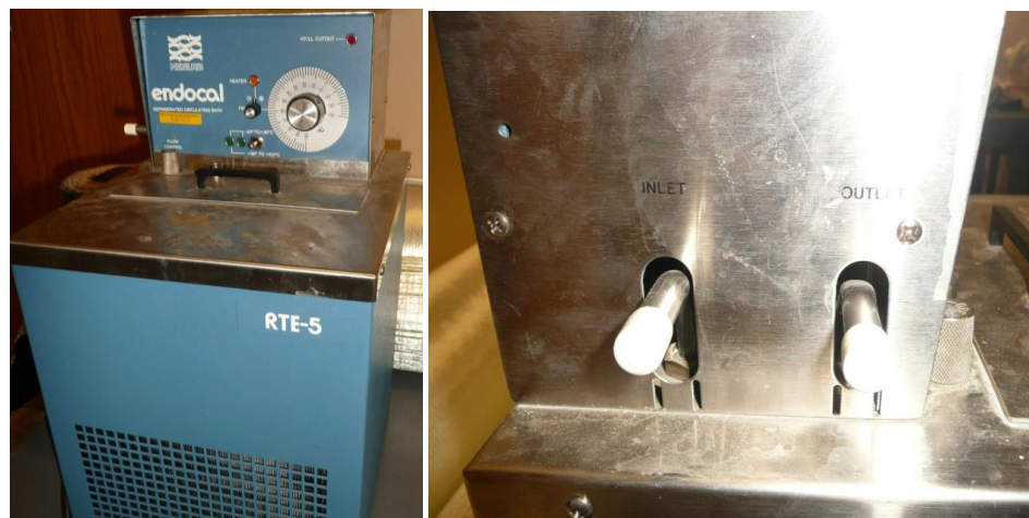
Figure 21: Endocal Refrigerated circulating bath.
