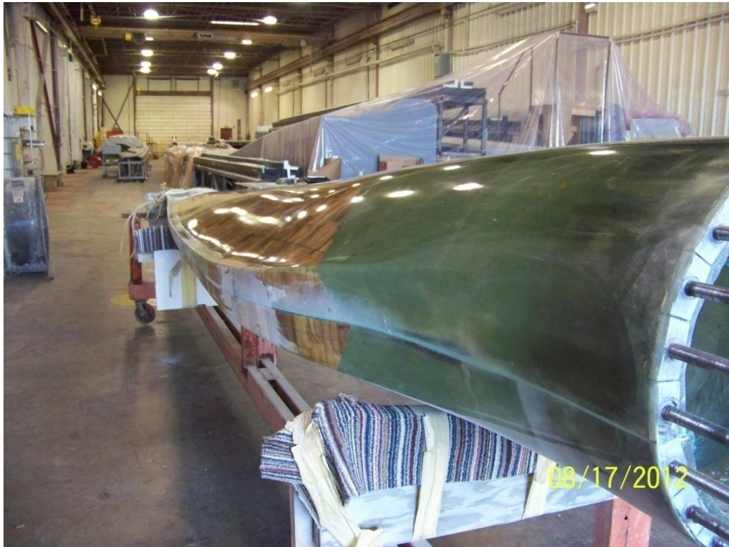
Figure 12: Completed blade manufactured at TPI.
