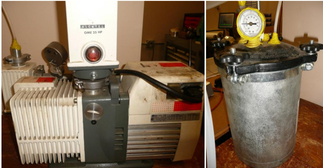
Figure 24: Alcatel Industrial vacuum pump and resin trap.
