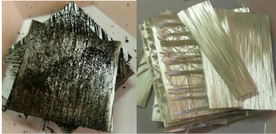
Figure 59: Fiber volume samples that were not burned off completely (left), and samples that were completely burned (right).
