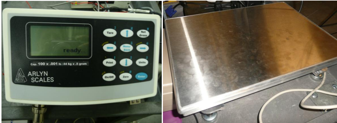
Figure 25: Arlyn Scale used to monitor flow rate. Left is control panel, right is measurement platform.
