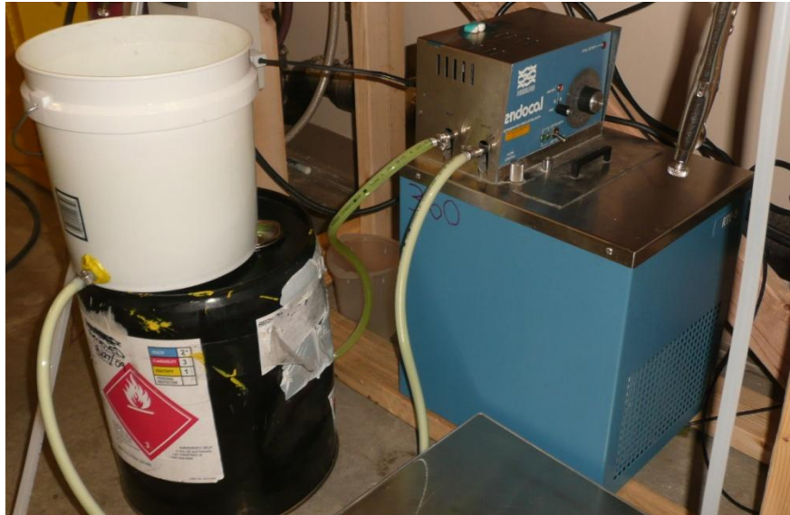
Figure 23: Endocal heater/chiller with heat transfer bucket and tubing attached.
