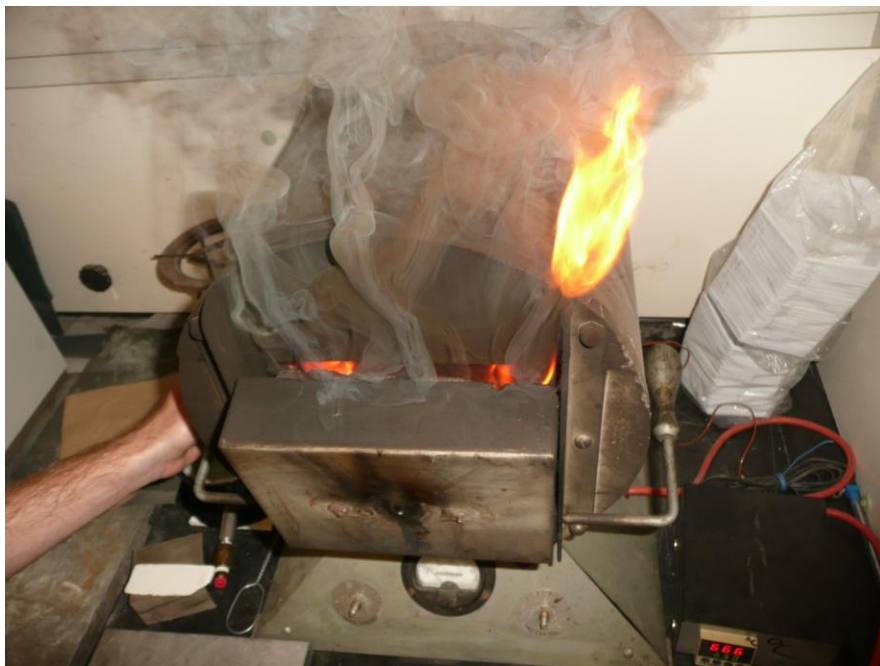
Figure 44: Burn-off test being performed in an electric oven at 650 °C.
