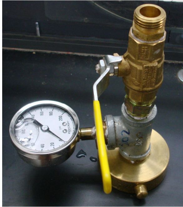
Figure 2.6 Hydrant Static Pressure Gauge
