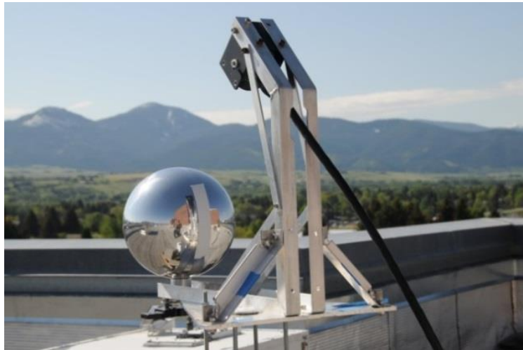
Figure 2-10. The dome all-sky ICI uses an aluminum dome to reflect the whole sky into a FLIR PathFindIR LWIR camera. The off-axis position of the camera is to avoid blocking the zenith sky (photo by Joe Shaw).
