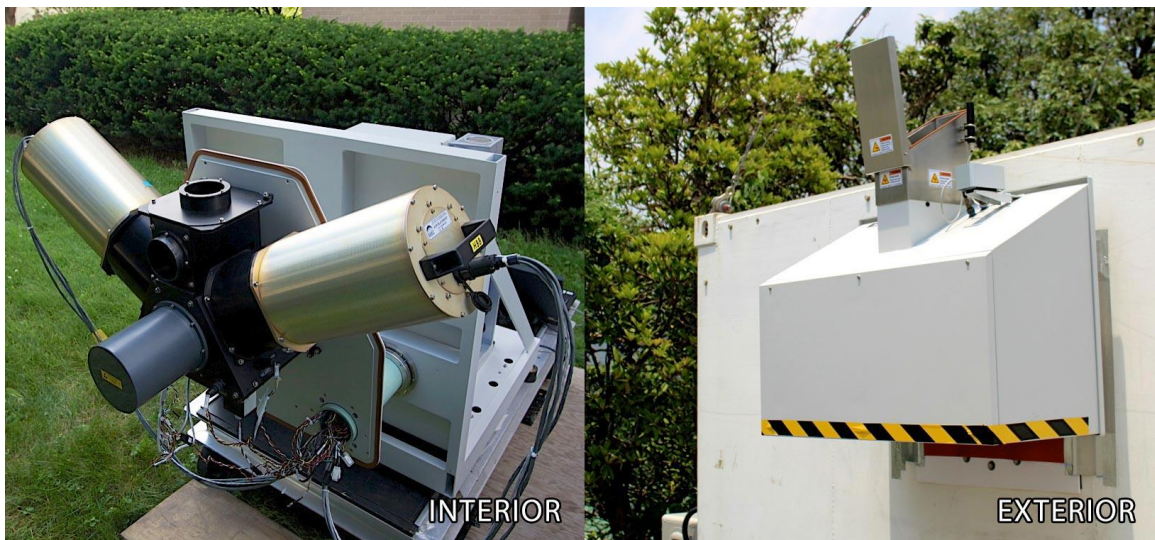
Figure 7-3. The Atmospheric Emitted Radiance Interferometer at the ARM Southern Great Plains Site; the ARM NSA site has a similar instrument. (Photo from arm.gov).
