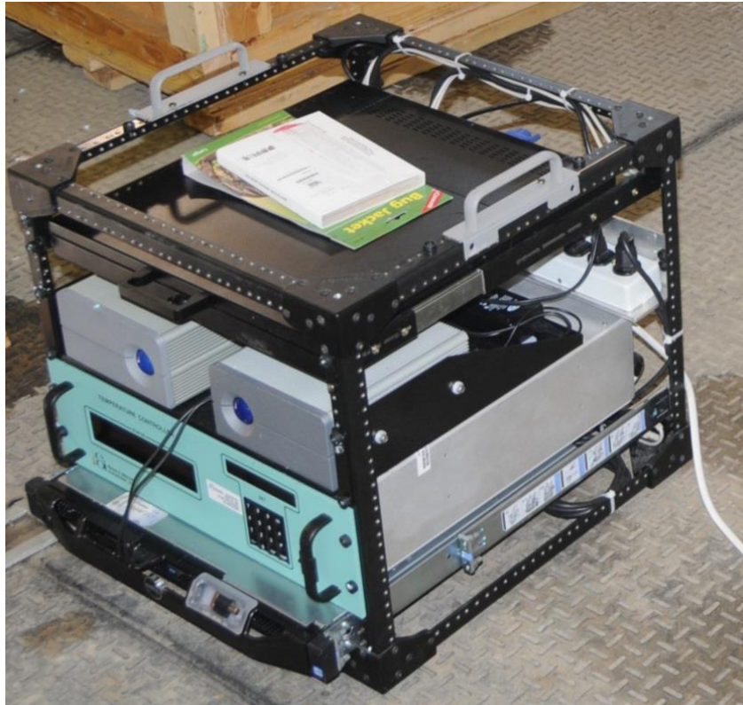
Figure 3-5. ICI electronics rack containing the computer, display, blackbody controller and two RAID external hard drives providing 1TB of redundant storage.
