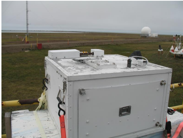
Figure 2-9. The ICI3 instrument during its deployment in Barrow, AK. The exterior paint on the instrument has been worn by the harsh Arctic environment.
