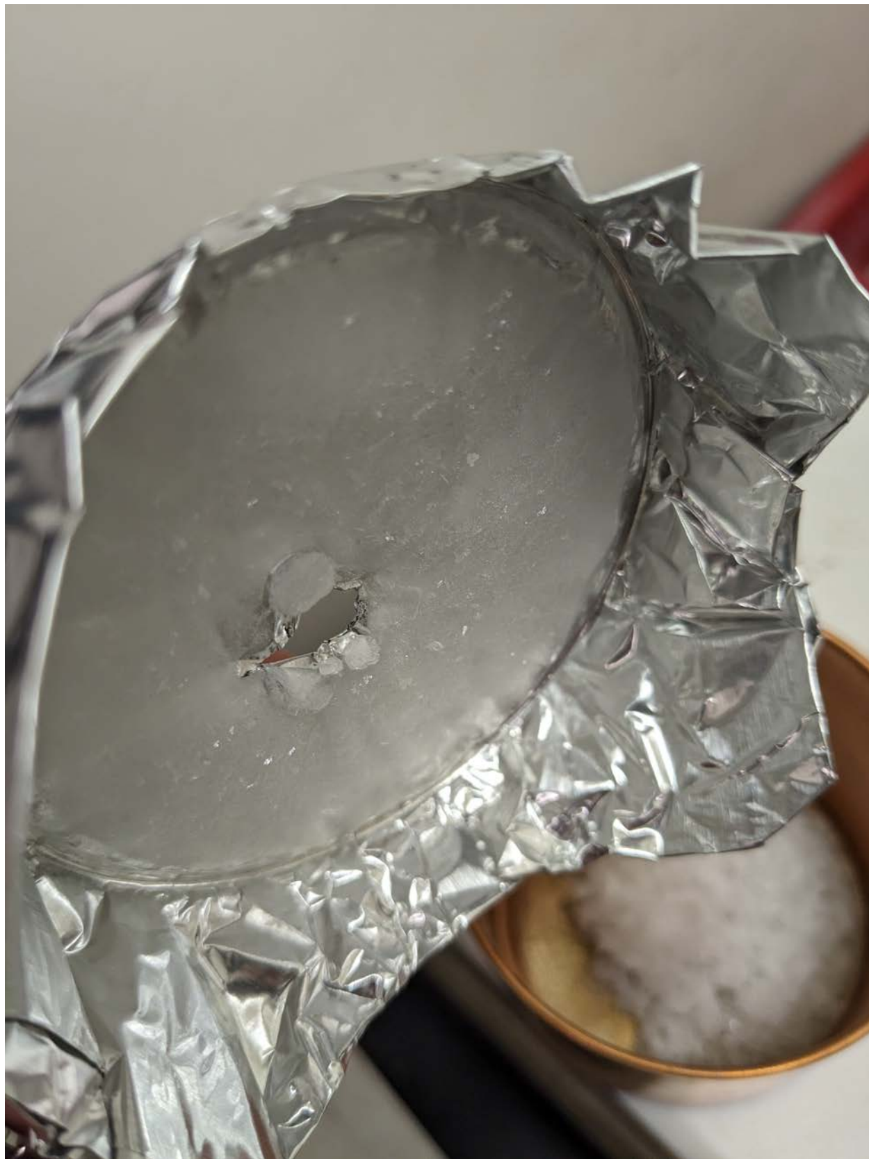
Figure 190: A thick layer of camphor that has formed on the inside of the Al-foil cover to the copper crucible used for camphor heating after many loading trials. It must be scraped off and re-crushed to produce a high-enough concentration of camphor in the beaker when heated.
