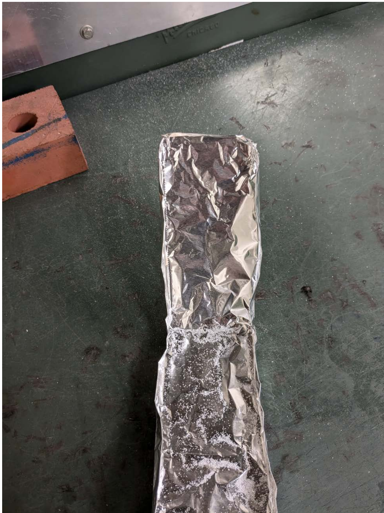
Figure 194: A photo of a piece of aluminum foil used to catch glass after it fell through the flame. Karger catching pieces may be beneficial, partly because many of the rounded particles tended to be found further from the flame, possibly due to a longer amount of time spent in the jet of hot air.
