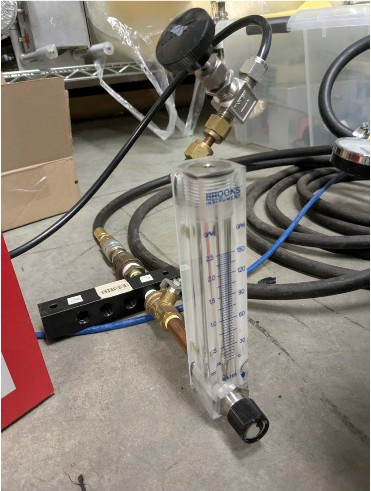
Figure 196: The flow meter used to determine the flow of air for the tumbler. It is designed to be used with water, but could in principle be calibrated to get an absolute measurement of the flow rate for air.
