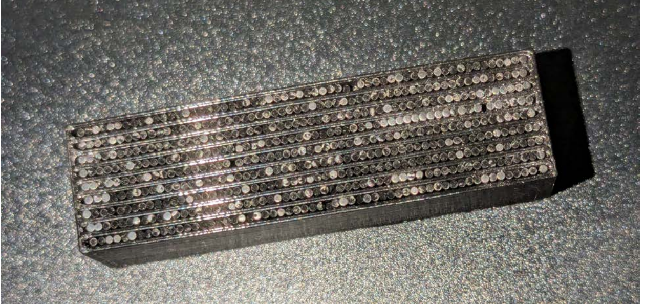
Figure 54: Pentel 0.5mm HB pencil lead packed by hand into a 9 slots for use in the TeachSpin magnetic susceptibility measuring kit. After packing, the ends of the lead were lapped smooth to try to keep the lengths as close to uniform as possible. Measurements of the susceptibility of the holder in both orientations were taken separately and subtracted off the results for the lead-packed holder.
