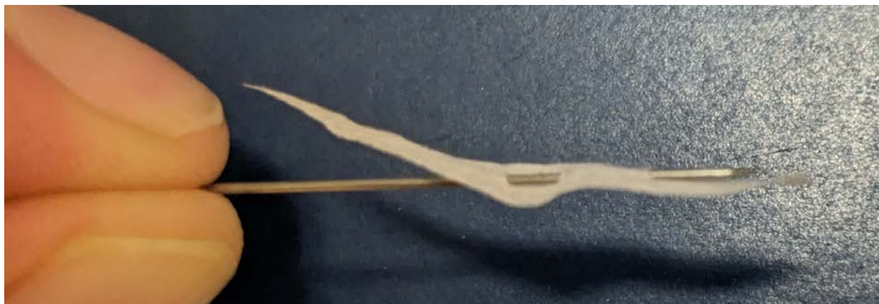
Figure 192: A piece of Kimwipe skewered on a SE-20T Signatone tungsten probe tip, used for cleaning debris off of pole pieces in magneto-gravitational traps.
