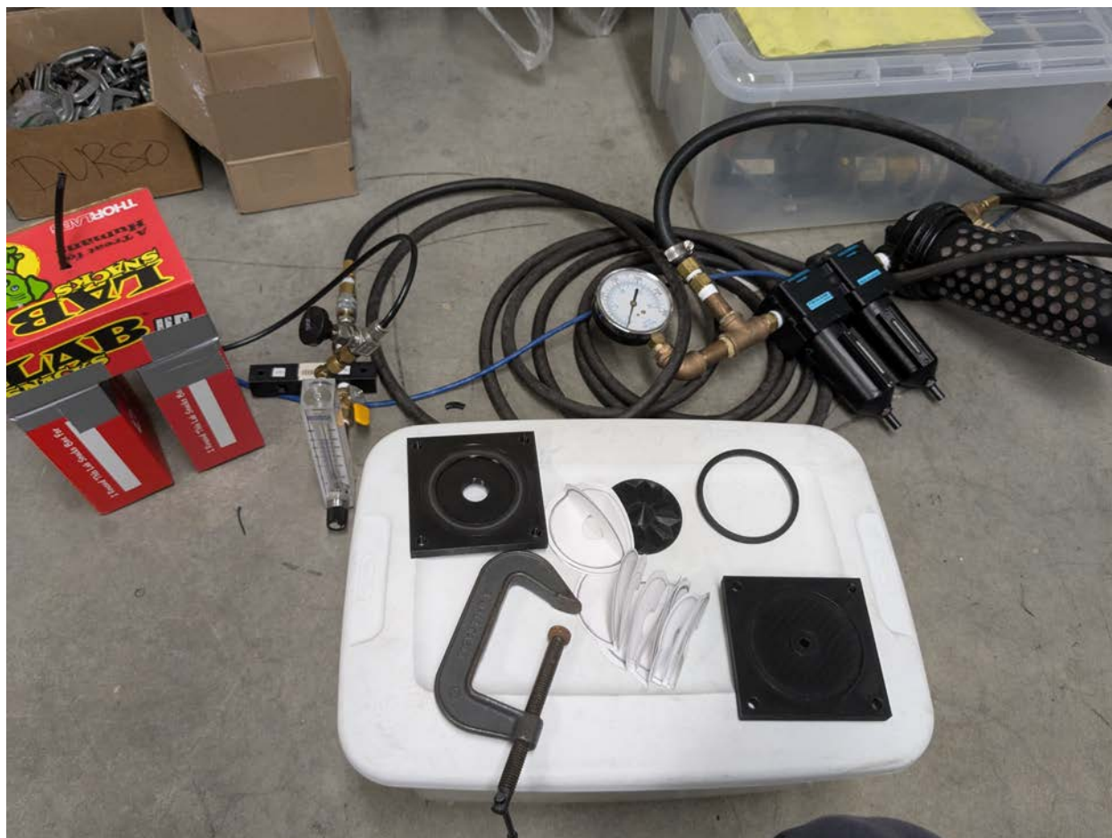
Figure 197: In image of the tumbler components disassembled. The taped-together Thorlabs boxes on the left hold the tumbler upright while the black tube is inserted through the hole in the bottom plate. The filters on the right help regulate pressure and keep the tumbler clean.
