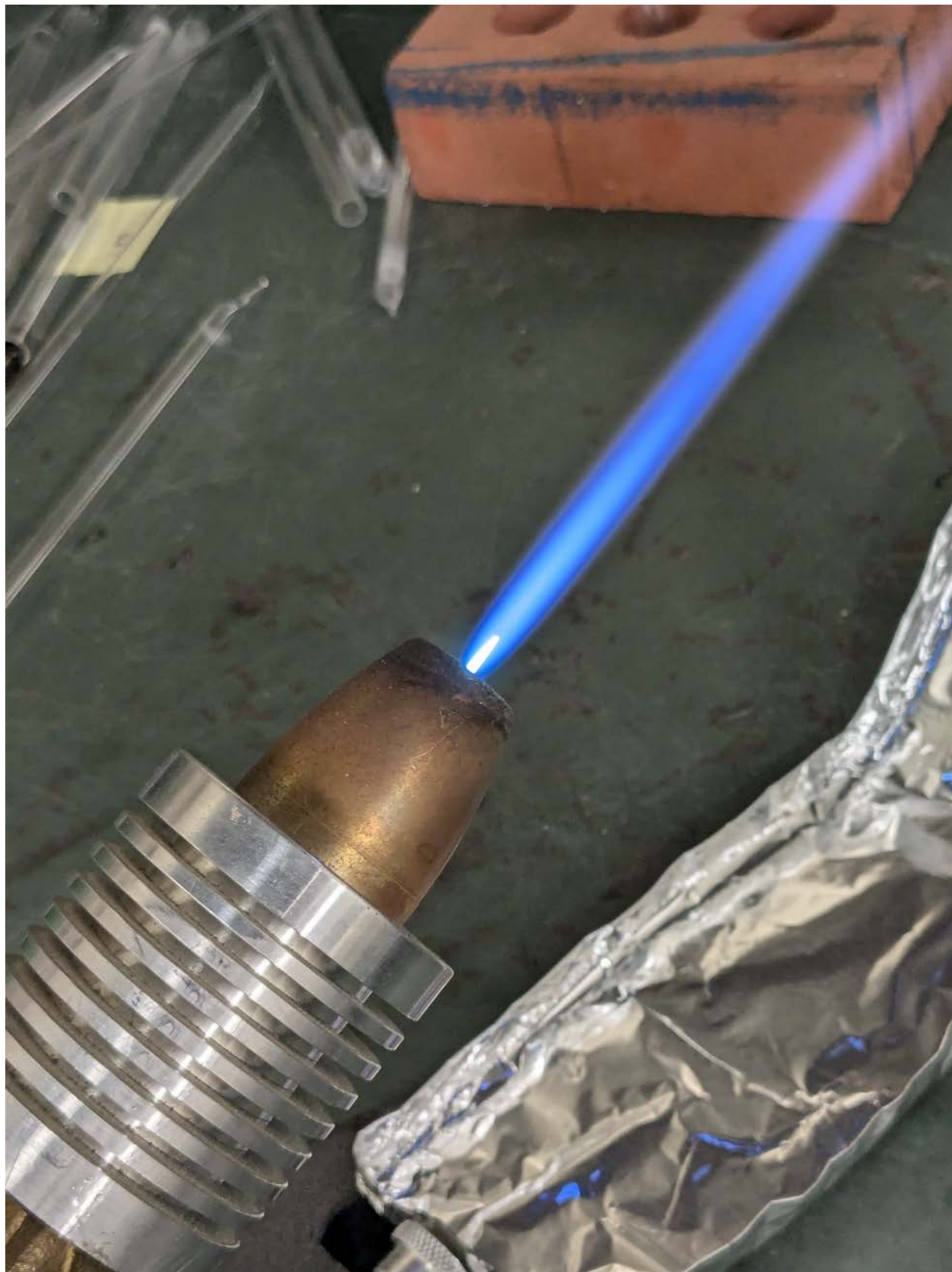
Figure 193: A photo of the type of flame used for flame spheroidization. Glass powder was dropped through the tip of the smaller, brighter blue flame at the center.
