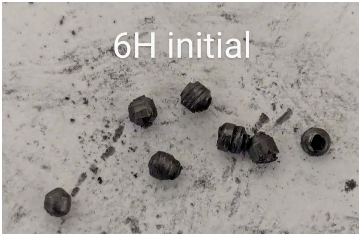
Figure 43: Pieces of 0.5mm Pentel 6H pencil lead, lathed on the Mini Milling Machine (KLUTCH 49657) by use of a tungsten carbide blade. Rough edges can be seen where the pieces broke off at their thinnest point during the lathing process.
