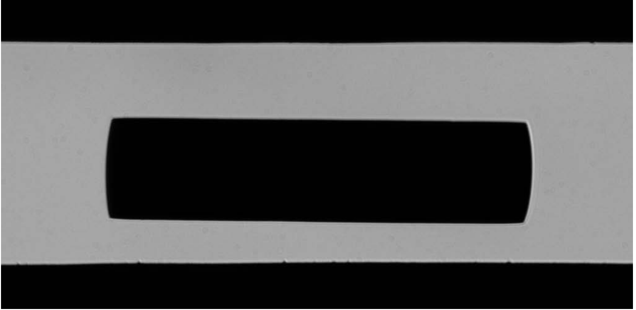
Figure 155: An image of Edwin (HB05-2.4-lapped) taken under UHV. The diameter of the particle is about 0.56 mm and the length is about 2.4 mm. The bottom and top black parts of the image are the silhouettes of the bottom and top pole pieces, respectively.
