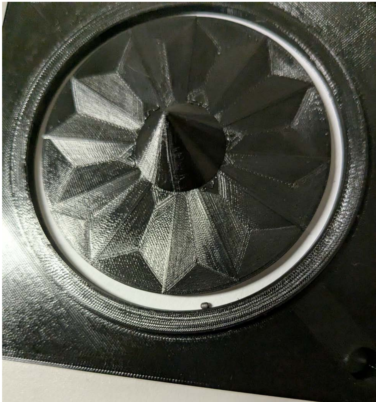
Figure 42: An image of the particle tumbler (printed from PETG with a 3 mm tumbling track) with a particle inside ready to be tumbled. The top plate is not shown. The conical shape at the center was designed to make 3D-printing the part possible without additional supports.
