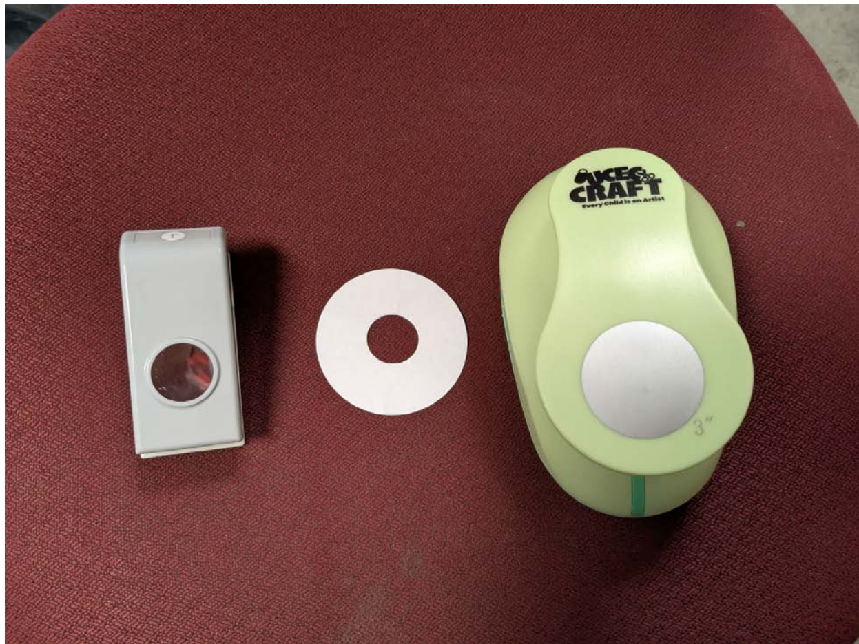
Figure 198: Photo of the hole punchers used to cutout pieces of printer paper for use in the pencil lead tumbler. The large green cutter is used first, then the piece is folded over and the gray cutter is used to cut out a half circle from the folded piece, which can then be unfolded.
