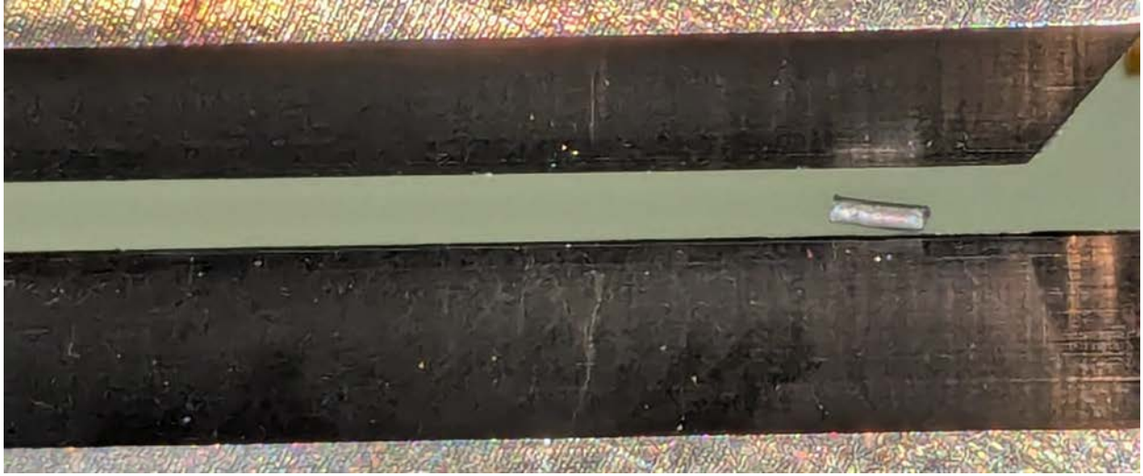
Figure 40: A piece of \sim 67\% graphite, \sim 33\% high-temperature epoxy (Epo-Tek 353ND) (by volume) graphite composite levitated in a Long MGT with end magnets, annealed Hiperco 50A pole pieces, and unshaved magnets. The graphite volume ratio of this particle slightly exceeds that of Pentel HB pencil lead, which has a volume ratio of about 51%, but levitates less well.
