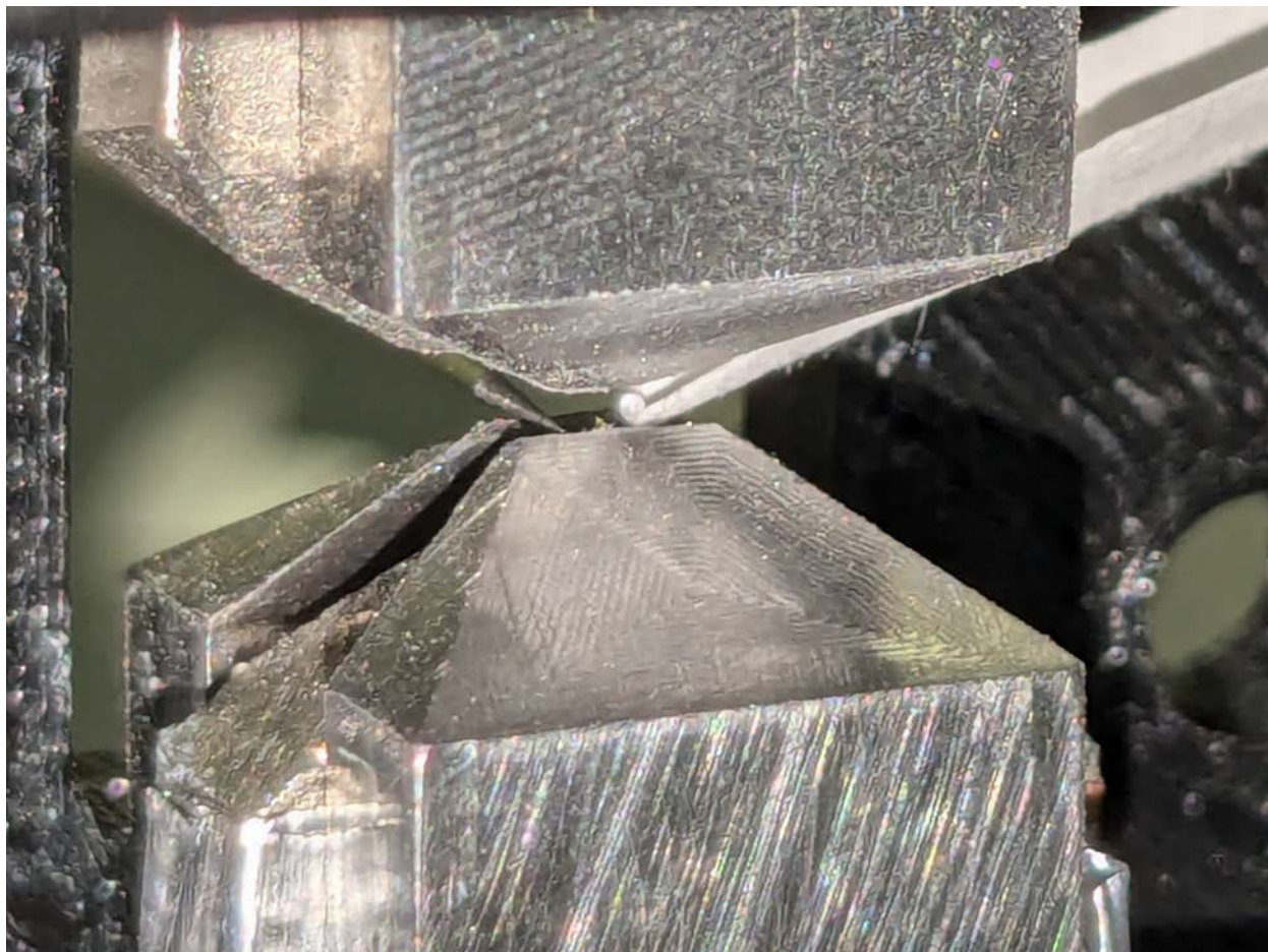
Figure 30: Image of a 300 \mu\text{m} sphere being loaded into a modified Short MGT . The paper could be gently jostled by hand to release the sphere, while the tungsten probe tip was placed to block its exit from the trap on the far side. The relatively large size of the sphere made it possible for small vibrations to overcome its contact force to other surfaces, allowing for this kind of release.
