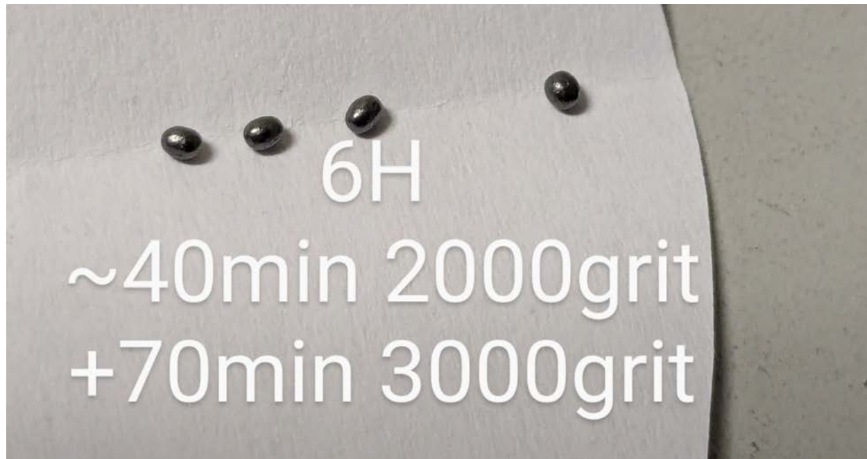
Figure 44: Pieces of 0.5mm Pentel 6H pencil lead tumbled in the particle tumbler for 40 minutes with 2000 grit silicon carbide sandpaper followed by 70 minutes using 3000 grit sandpaper (flow rate not well-controlled or documented). Note the slightly oblong shape and smooth surface finish.
