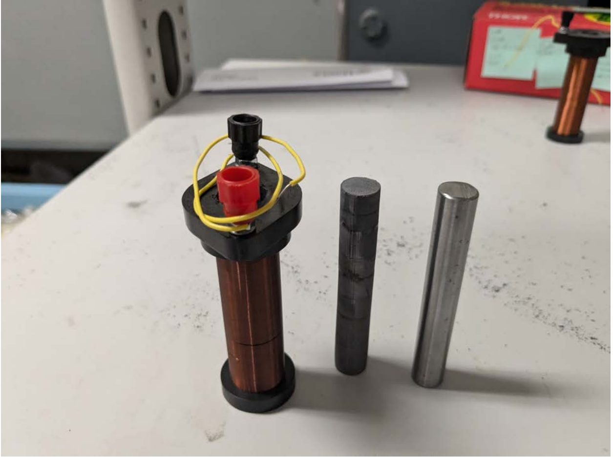
Figure 16: Left: Inductor used to measure the loss of the metal rods – 260 turns, A_{cc} = 1.1 \text{ cm}^2 core cross-sectional area, length 8.6 cm. Middle: Hiperco-epoxy composite rod – broken pieces were fit back together using high-temperature epoxy (Epo-Tek 353ND) . A small current could still be passed through the length of the rod, indicating at least a partial electrical connection throughout its length. Right: A solid rod of Hiperco 50A prior to in-house annealing.
