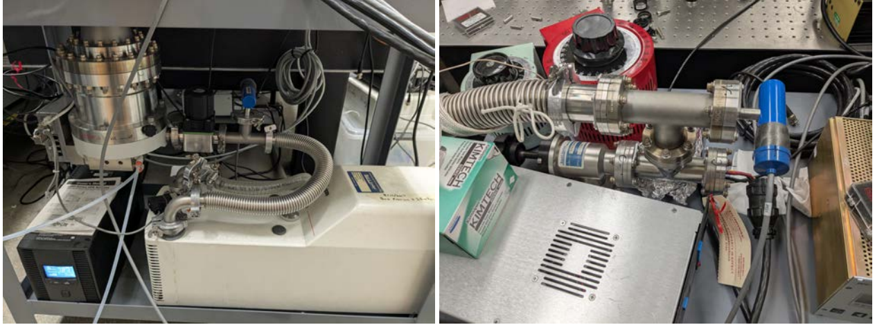
Figure 13: Left: Photo of the rough pump/turbo pump setup for the Short MGT vacuum chamber. Right: Photo of the top of the table containing the vacuum gauges and bellows connection to the chamber.
