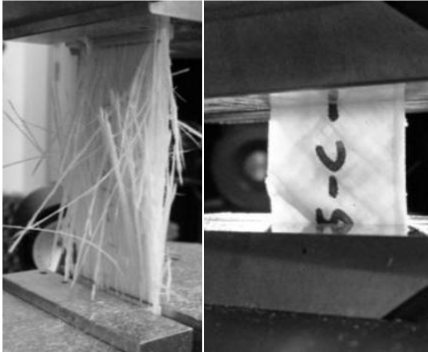
Figure 52: Representative failed coupons in machine grips.
