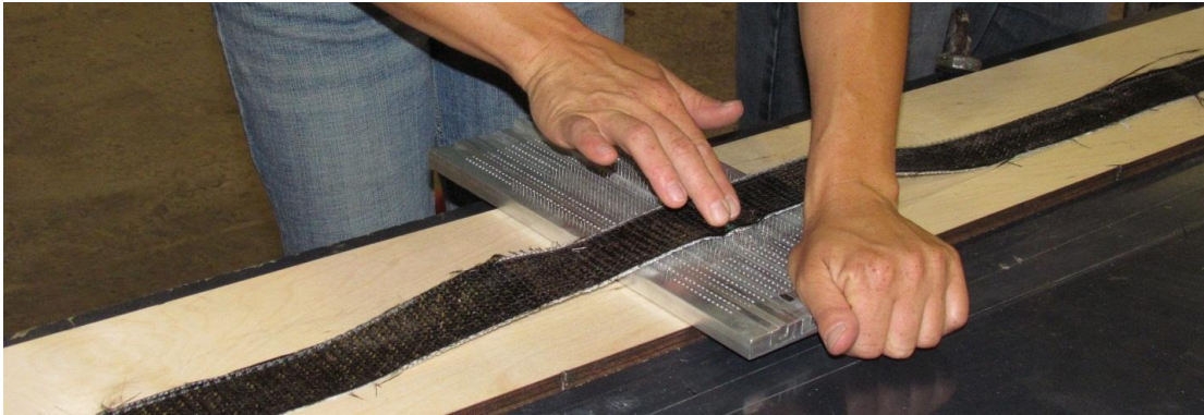
Figure 92: Photo showing IP waves formed into one carbon laminate of the spar cap
