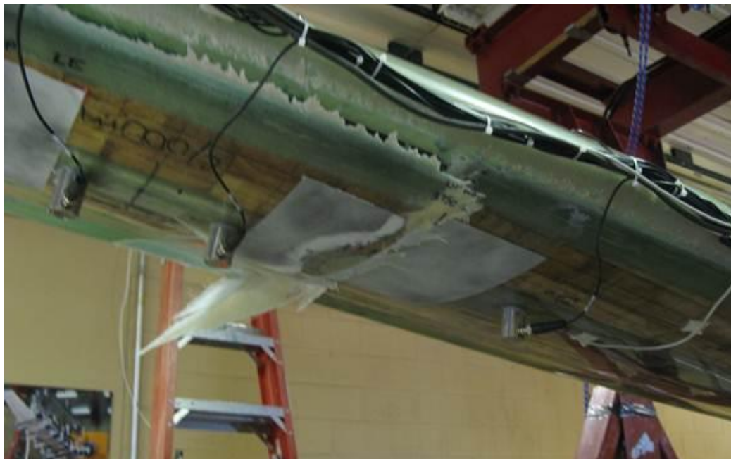
Figure 104: OP Wave failure at the 3.75m HP location
