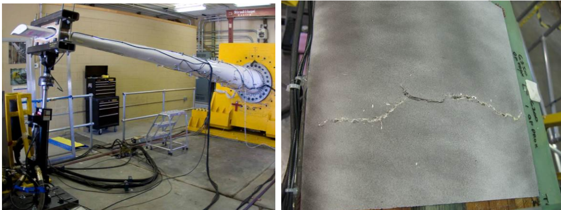
Figure 82: Blade test (left), Failure at flaw location (right)
