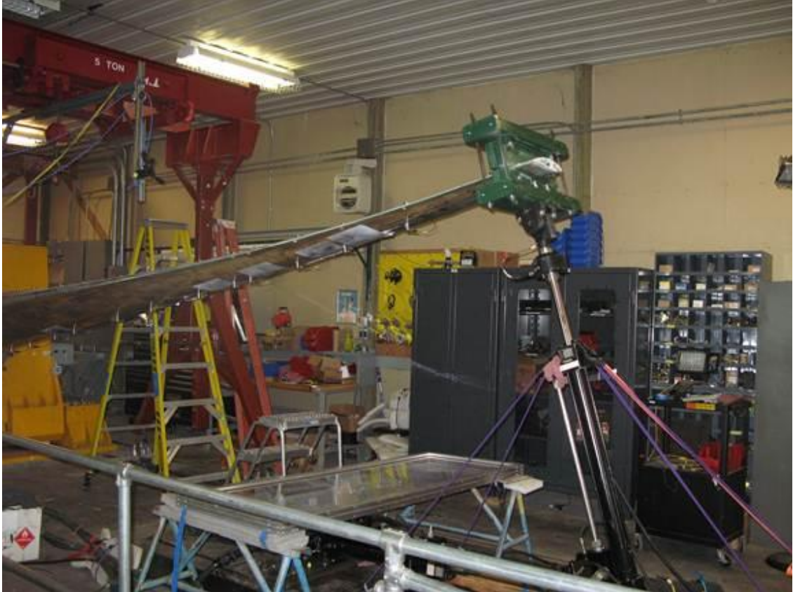
Figure 100: Fatigue test at the 7m station
