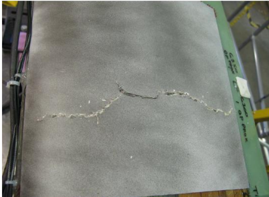
Figure 103: OP Proximity Wave failure at the 6.2m LP location
