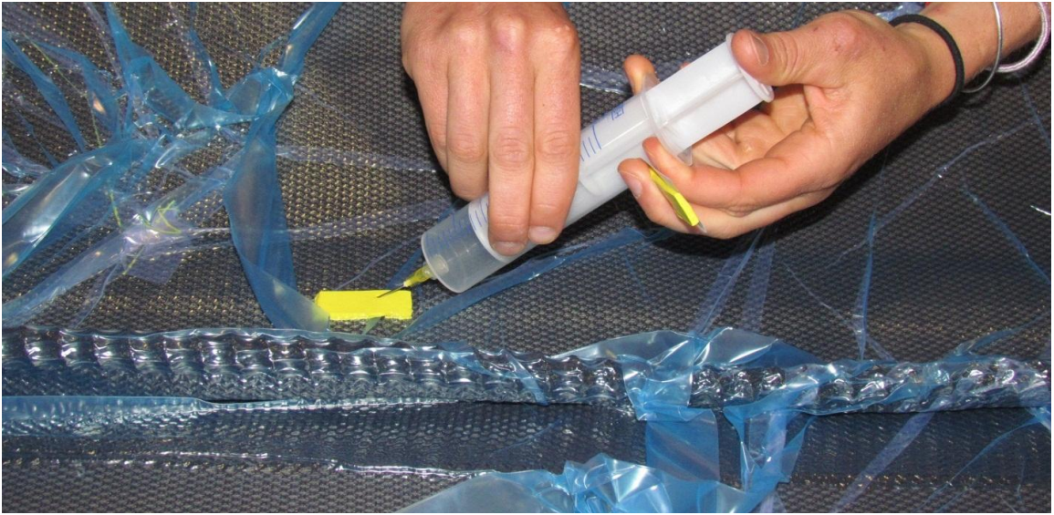
Figure 99: Injection of air to generate porosity in a partially cured skin.
