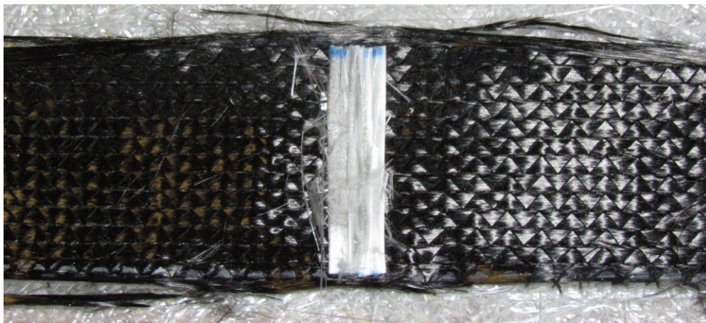
Figure 97: Photo showing a stack of glass fibers that will create one OP wave.
