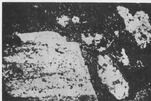
Figure 2. Photomicrograph in polarized light basic porphyry, Fort Ellis subarea. Large grains are plagioclase phenocrysts.
