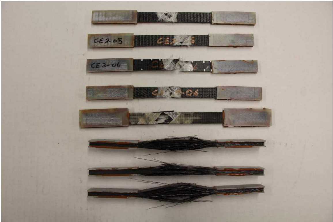
Figure 26: Examples of failed coupons of MHK study materials (J6-8 & CE1-5) showing typical failure modes
