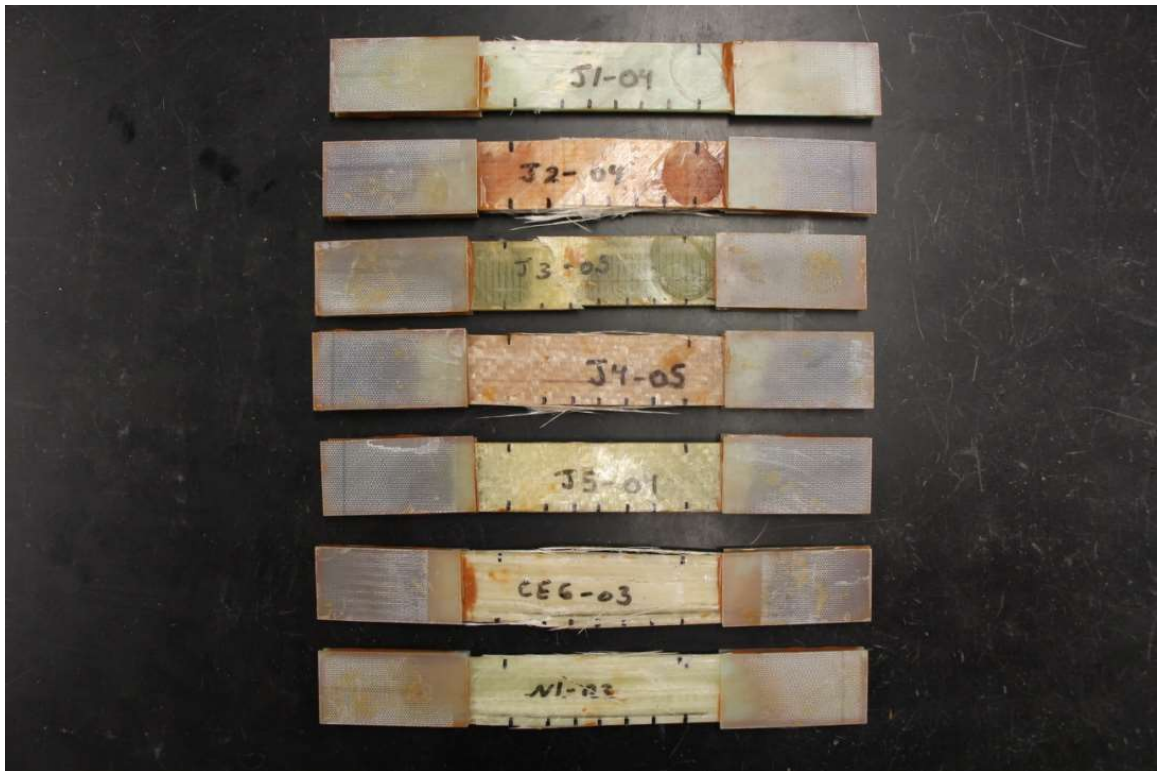
Figure 25: Examples of failed coupons of MHK study materials (J1-5, CE6, & N1) showing typical failure modes
