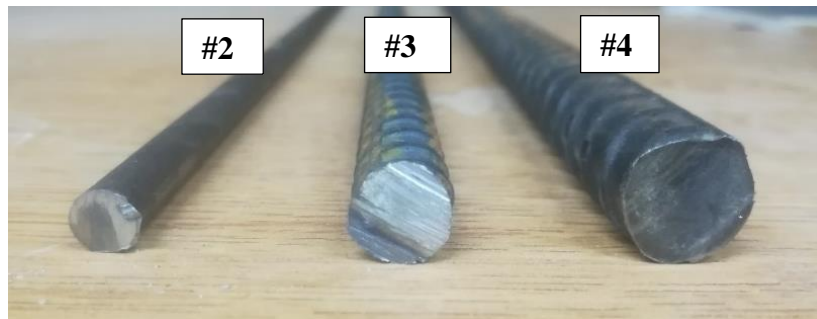
Figure 8. Rebar used in this study.
