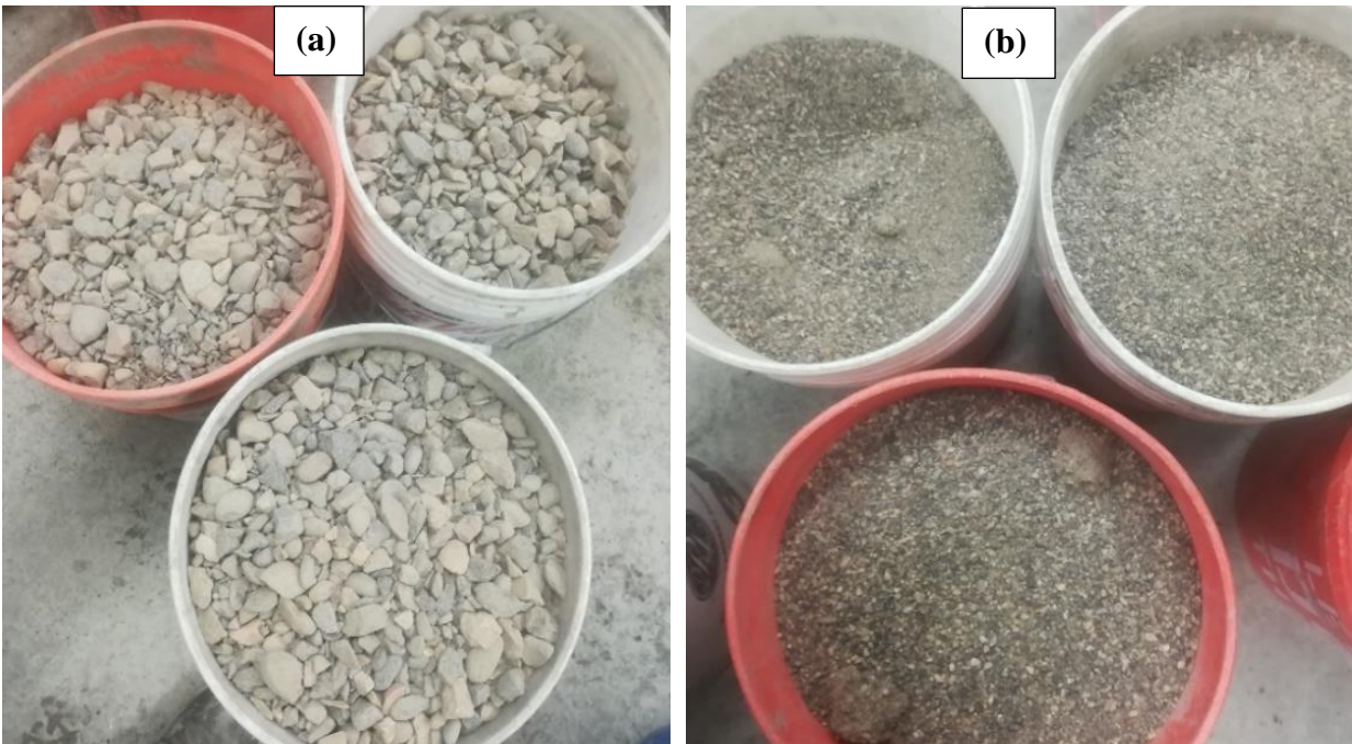
Figure 7. (a) Coarse aggregate, (b) Fine aggregate.
