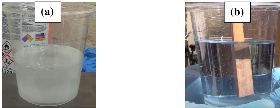
Figure 50. Epoxy resin; (a) Crystallized, (b) After removing crystallization. (Andrés Chavarria YouTube channel).
