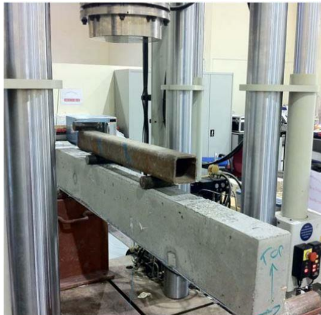
Figure 6. Four-point bending test set up used by Hawileh et al. (2014).
