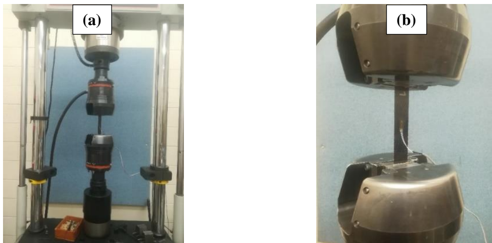
Figure 16. Experimental setup of FRP coupons; (a) Example coupon, (b) Zoomed in photograph of example coupon with strain gauge attached.
