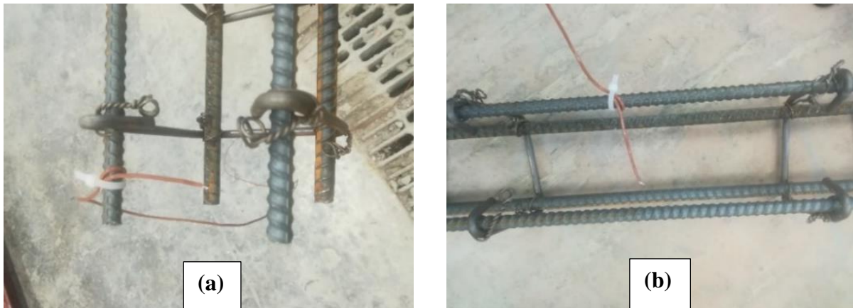
Figure 20. Thermocouple; (a) At the edge, (b) At the middle.
