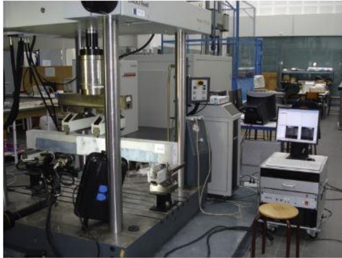
Figure 5. Four-point bending test set up used by Attari et al. (2012).
