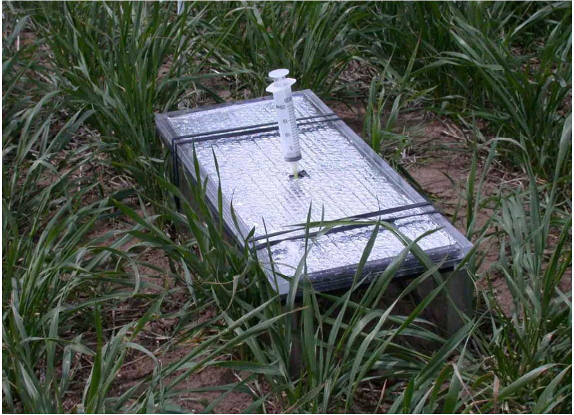
Figure 9. Vented chamber placed between crop rows of a continuous wheat rotation. Chambers were sealed during gas sampling with an insulated cover.
