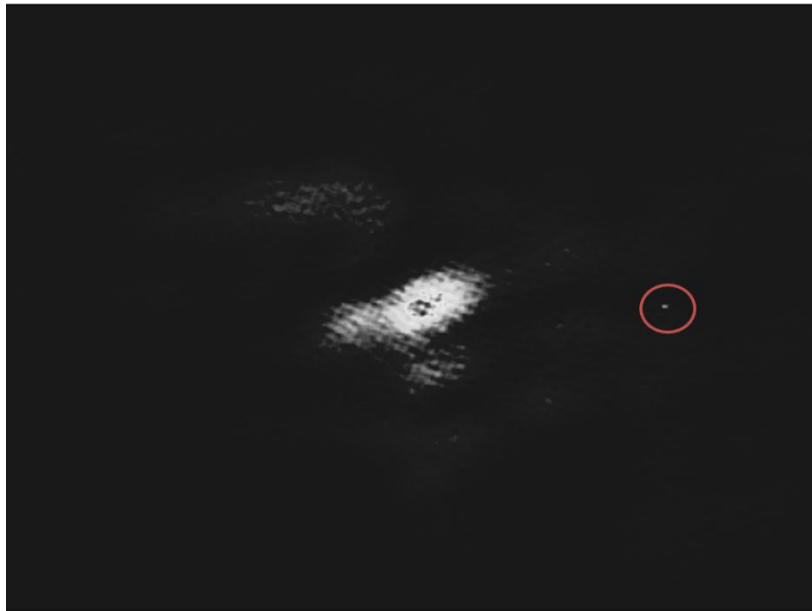
Figure 46 The correlation between two pupils. The offset is the bright point contained in the red circle. This offset from center was used to place the pupil in the mosaic.
