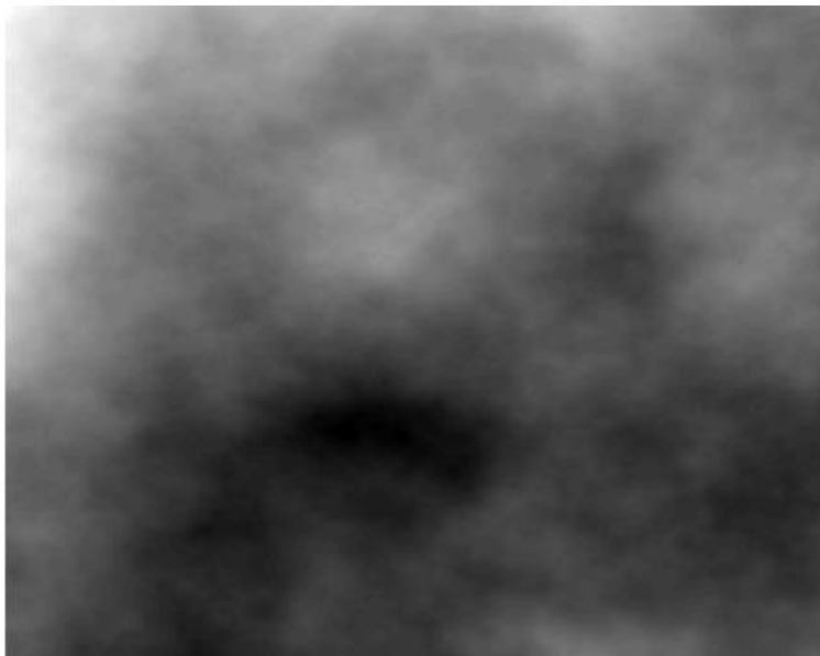
Figure 15 The phase screen acting as a model for turbulence. The cloud-like nature of turbulence is clearly visible here.
