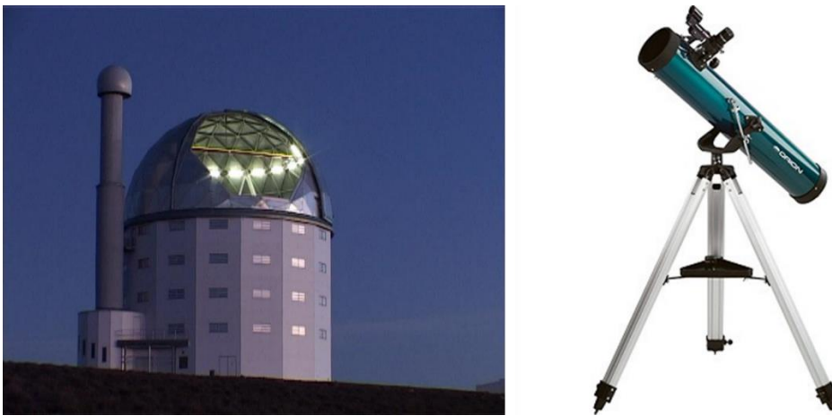
Figure 2 The Salt [2] and the Orion telescope [3] used to illustrate how the difference in aperture size is the main reason that their resolutions are so different.
