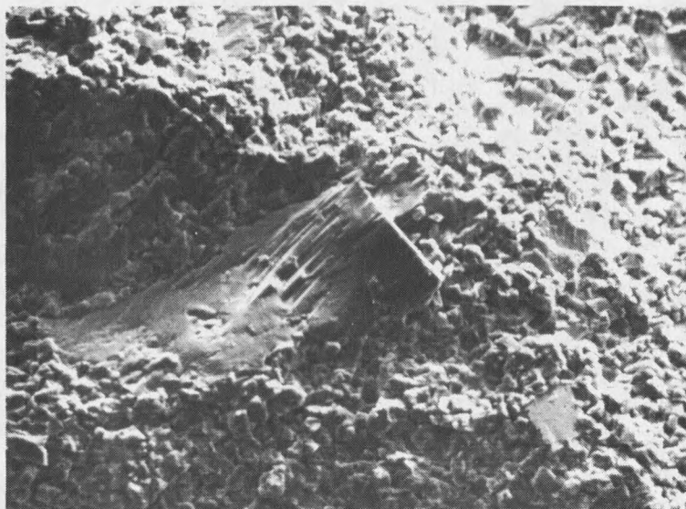
Figure 10. Typical LF-1 crystal textures. A. Very finely crystalline matrix and discoidal anhydrite. B. Anhydrite lath with parallel extinction. C. SEM photograph. An = anhydrite, D = dolomite. See text for complete descriptions.
