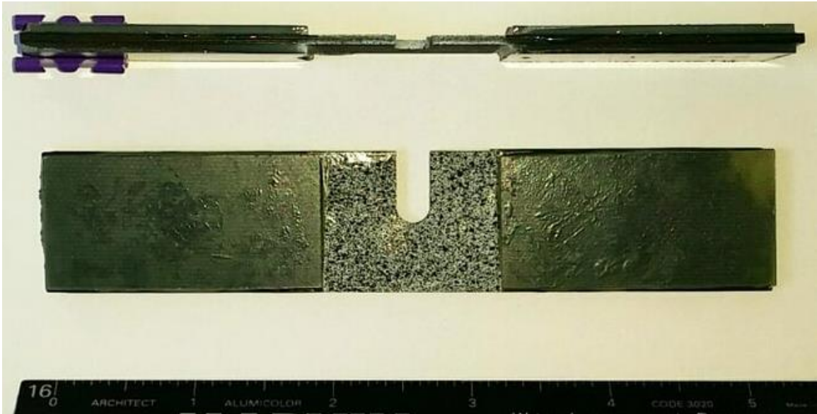
Figure 16. Result of manufacturing procedure. *This sample was flawed due to improper tabbing and was therefore not tested. A side-view to show tabs (top). Front view (middle). Inch ruler for scale (bottom)
