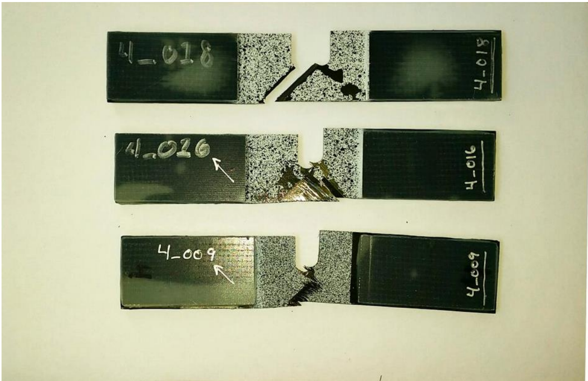
Figure 25. Laminate 4 interesting failures. Written labels correspond directly to the test matrix. For scale, coupon widths are 1 inch or refer to Figure 14 above
