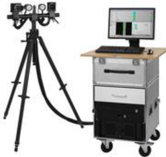
Figure 13. GOM ARAMIS hardware as shown in ARAMIS Manual [17]
