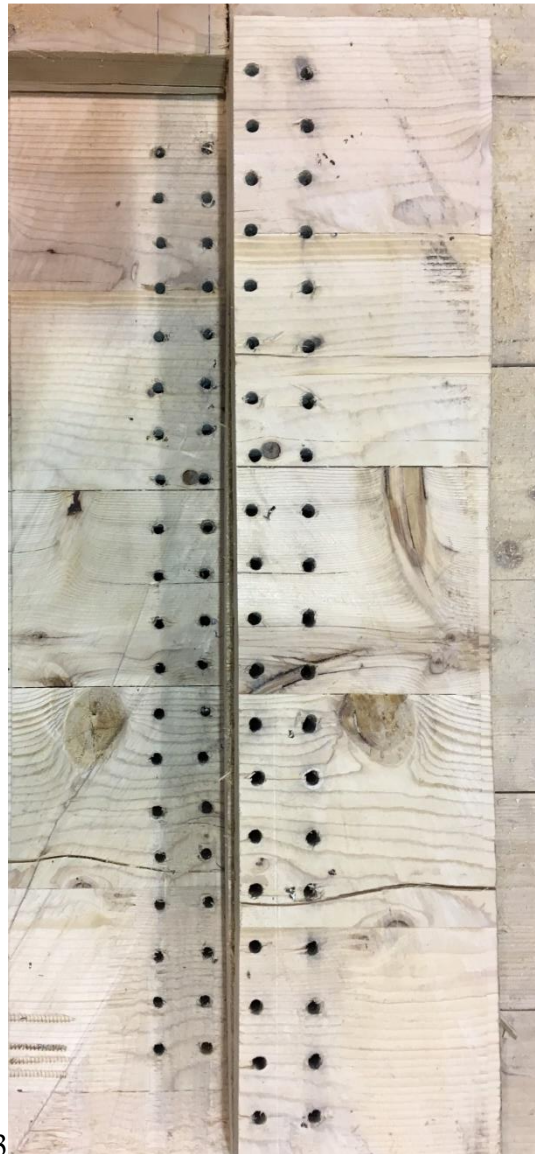
Figure 55 Tested CLT panel fastener holes
