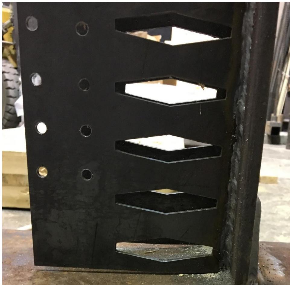
Figure 53 Tested full-scale reduced section knife plate
