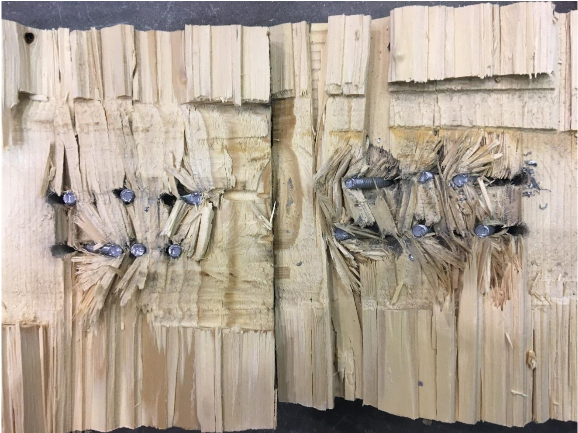
Figure 40 Single knife plate group fastener failure
