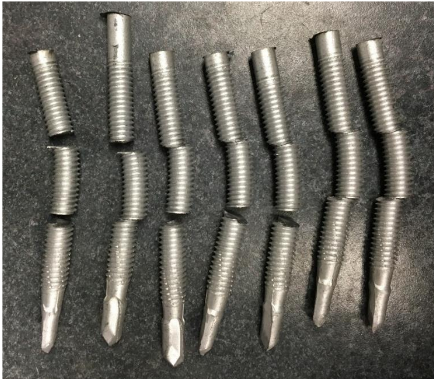
Figure 35 SDD shear failure
