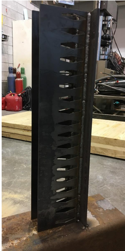
Figure 28 Full-scale holdown assembly
