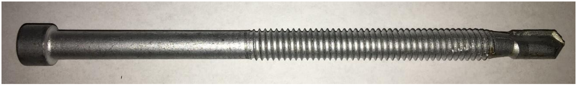
Figure 54 Tested shear wall fastener
