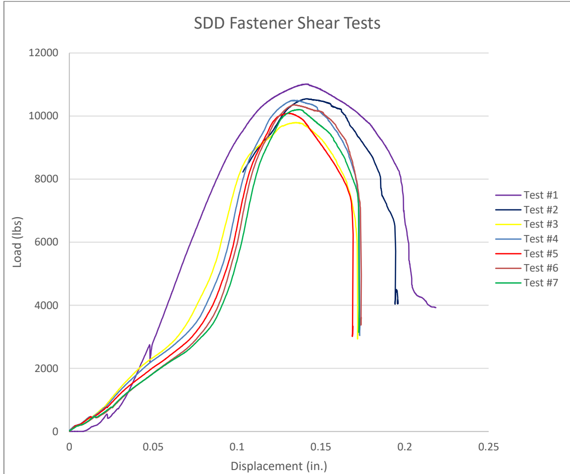
Figure 34 SDD shear test load-displacement
