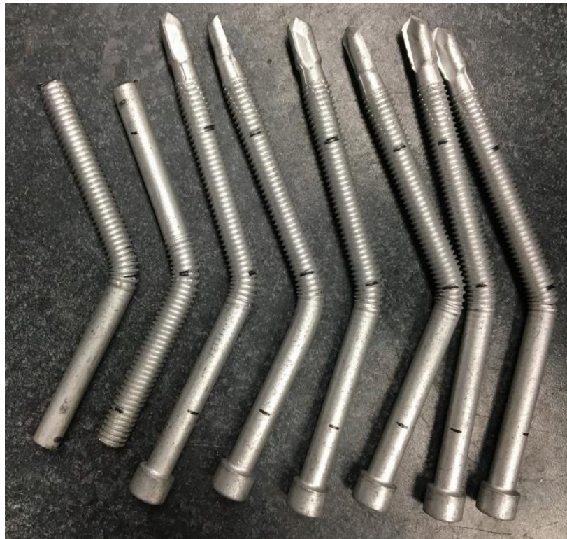
Figure 33 SDD bending failure
