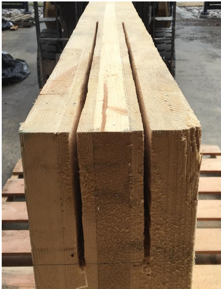
Figure 27 Full-scale knife plate slots
