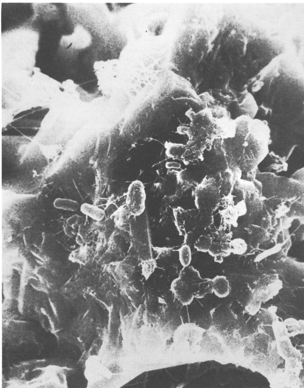
Fig. 1. Scanning electron micrograph of the pellet interior. The nominal pellet pore size is approx. 20\ \mu\text{m} .
