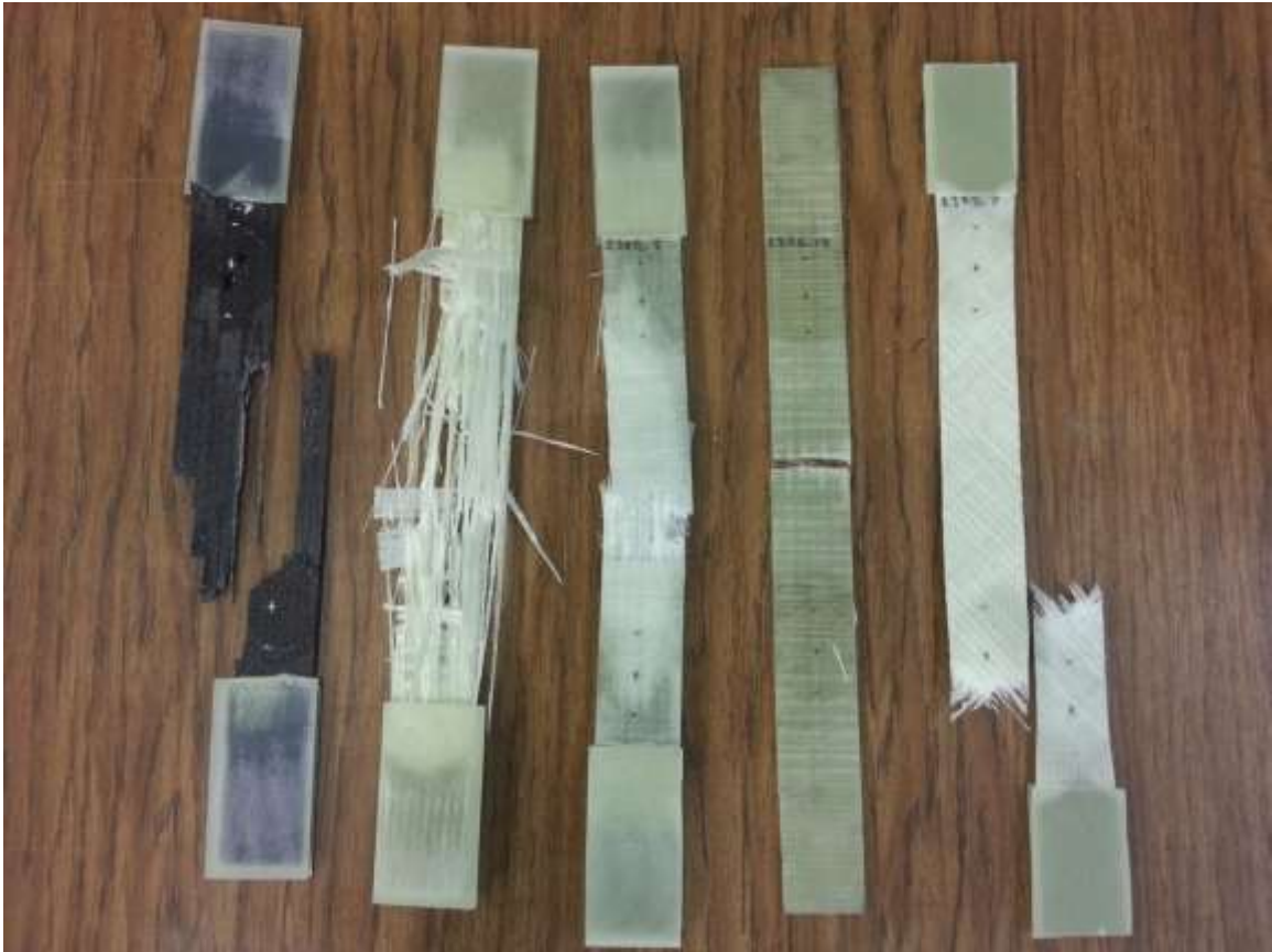
Figure 21: Various Failed Coupons from Left to Right: [0]_n Carbon-D and Glass-B, [90/0]_s Glass-A, [90]_n Glass-A and [45]_4 Glass-C
