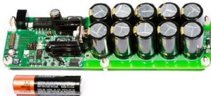
Figure 34. Picture of the PLD-200-ULW current driver used to drive the diode stack necessary for diode pumping the Monoblock pump laser.
