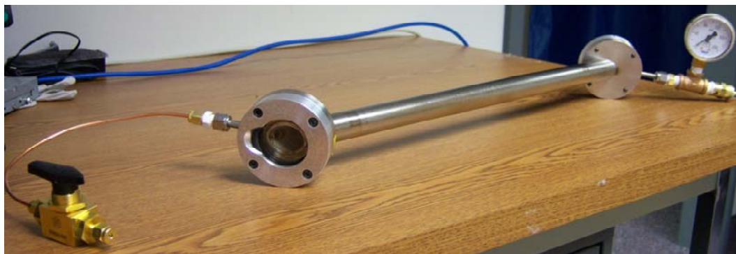
Figure 49. Constructed gas cell with additional components to fill the cell with \text{CO}_2 and safely monitor the pressure inside of the cell.
