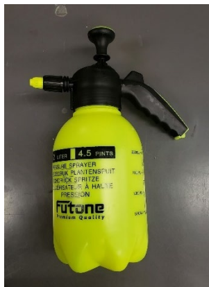
Figure 7 – Pump sprayer that was used to add moisture to sample to test moisture content effects on puncture resistance
