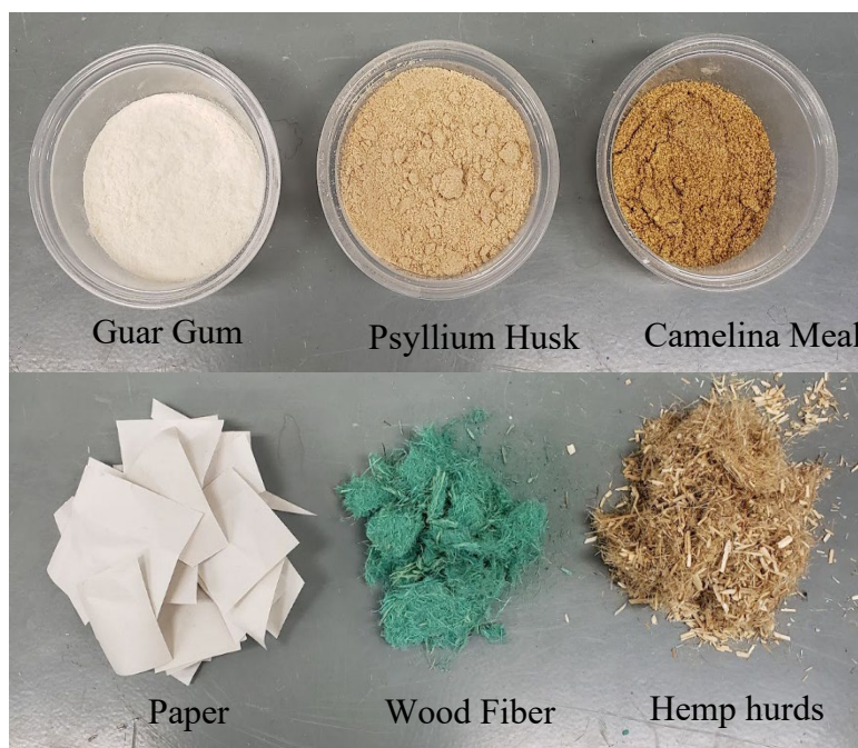
Figure 1 – Materials used as tackifiers in the different HM formulations (top) and fibrous materials used (bottom)
