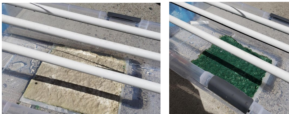
Figure 8 – Paper and wood sample after one min of a 15 min rain fastness test
