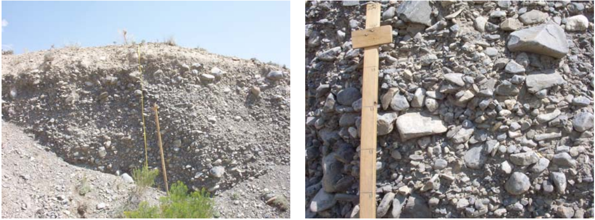
Figure 27. (A) Outcrop photo of Section 7. Jacob staff is 1.5 m high. (B) Close up photo showing the cobble gravel facies and the better sorted pebble gravel facies.
