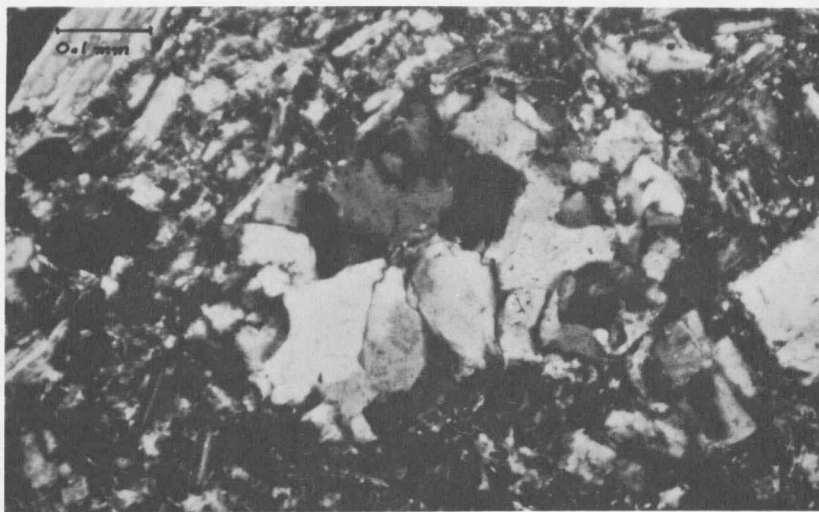
Figure 20. Photomicrograph of quartz aggregates in the groundmass of the southern Moose Creek intrusive. X-nichols.
