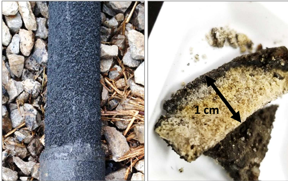
438 439 Figure 6. Mineral precipitation was observed on the downhole tubing following completion of the field 440 demonstration, visible as the bumpy coating on the perforated pup joint (left). The outer surface was 441 darker in color than the inner regions of the precipitate (right), perhaps due to exposure to wellbore fluids 442 following the field demonstration.
