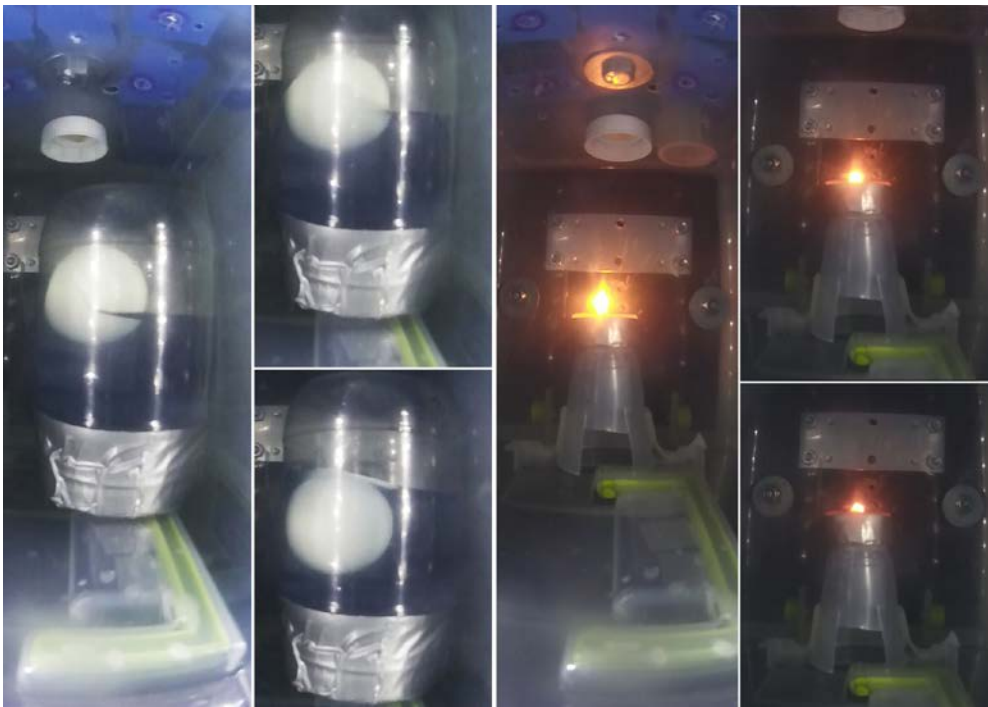
Figure 5. Detail views of a ping pong ball floating in water (left) and a candle flame (right) at T-1 second, T=0, and T+0.25 second of free-fall.
