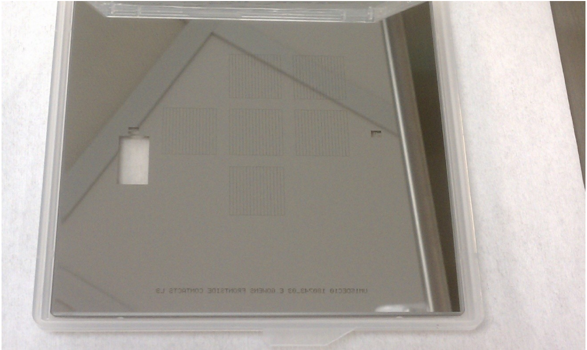
Figure C.3 A picture of Mask #3. The back side P+ barriers
