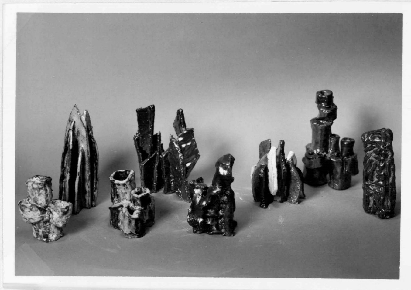
Figure 1. (left to right) A. Stoneware and 50% Compressed Shredded Paper, B. Stoneware and 50% Vermiculite, C. Stoneware and 25% Coarse Grog, D. Stoneware and 50% Sawdust, E. Earthenware and 50% Sawdust, F. Earthenware and 25% Coarse Grog, G. Earthenware and 50% Loose Shredded Paper, H. Earthenware and 50% Compressed Shredded Paper
