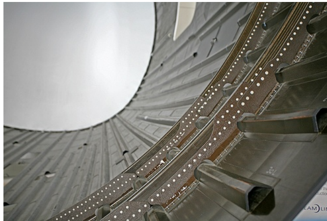
Figure 3: A one piece barrel section of the 787 Dreamliner fuselage. Using a one piece structure for the fuselage saves 40,000 to 50,000 fasteners.[10]
