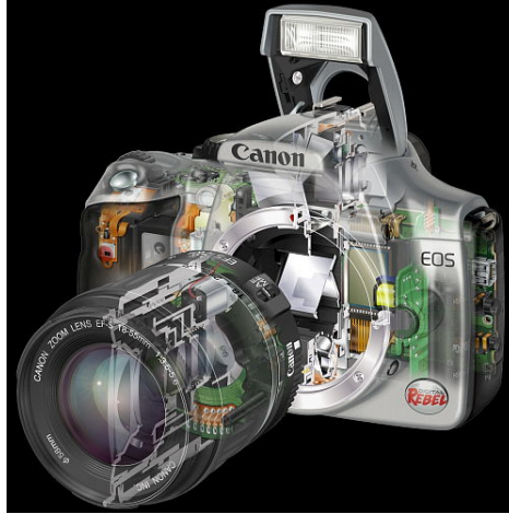
Figure 12: A cutaway view of the canon Digital Rebel 300d [3]
